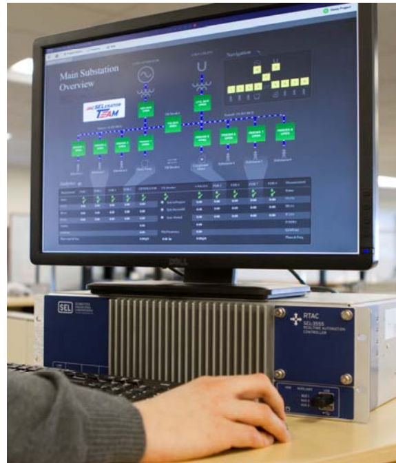
Integrated video port on the SEL-3555 RTAC provides localized HMI views.
