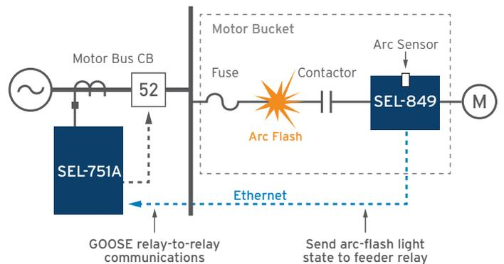
SEL AFD combines light-sensing technology with fast overcurrent protection.
