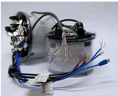
Figure 1 Example socket meter with pigtailed
