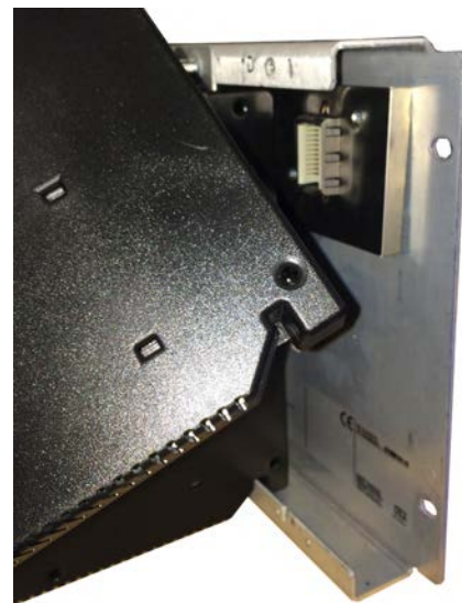
Figure 2 Notch for Module Alignment
