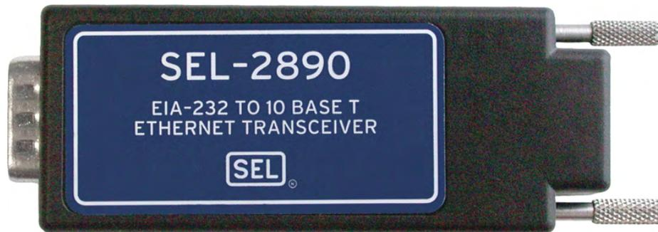
The SEL-2890 Ethernet Transceiver is an EIA-232 serial-to-10BASE-T converter. The SEL-2890 is powered by 5 Vdc provided on Pin 1 of the serial communications ports on most SEL devices. Convert existing SEL products to Ethernet capability simply by using the SEL-2890.
