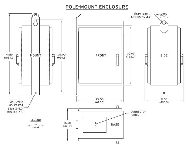
Figure 16 SEL-651R Dimensions and Mounting Drill Plan (Dual-Door Enclosure)
