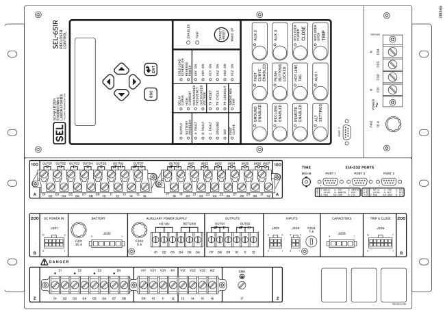
Figure 12 Front View of SEL-651R Modules (Single-Door Enclosure
