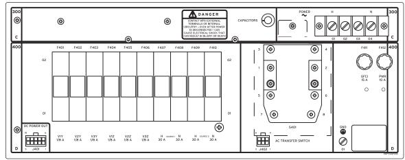
Shown fully equipped with fuse blocks and ac transfer switch.
