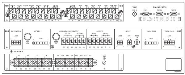
Figure 14 Rear View of SEL-651R Relay Module
