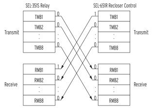
Figure 10 MIRRORED BITS Transmit and Receive Bits
