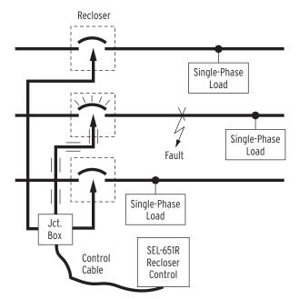
Figure 3 Single-Phase Tripping Isolates Only the Faulted Phase
