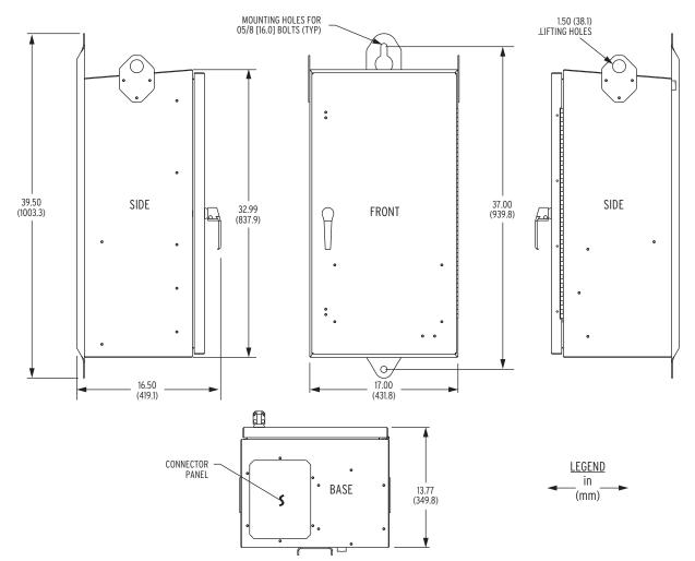
Figure 17 SEL-651R Dimensions and Mounting Drill Plan (Single-Door Enclosure)
