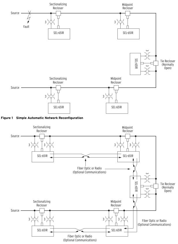
Figure 2 Advanced Automatic Network Reconfiguration
