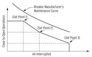
Figure 13 Recloser Contact Wear Curve and Settings
