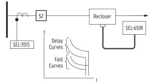
Figure 7 Coordinate the SEL-651R With Other Devices
