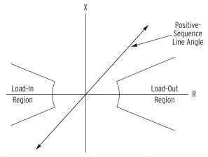
Figure 8 Load-Encroachment Logic Defines Load Zones (No Trip Zones)
