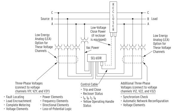
Figure 5 Connect Three-Phase Load and Source Voltages to SEL-651R
