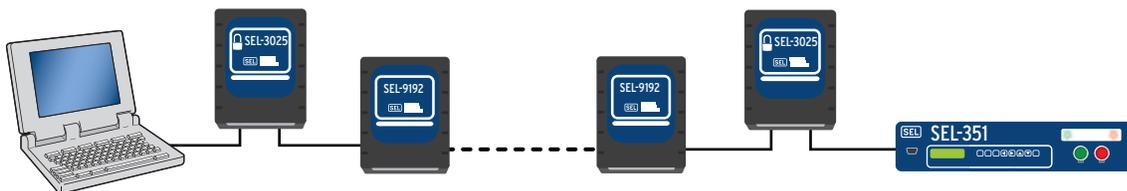
**Figure 3 Secure Dial-up Engineering Access Channel**
