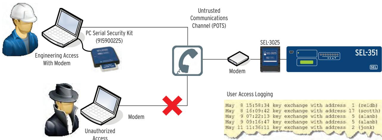
**Figure 3 Secure SCADA Communications Channel**
