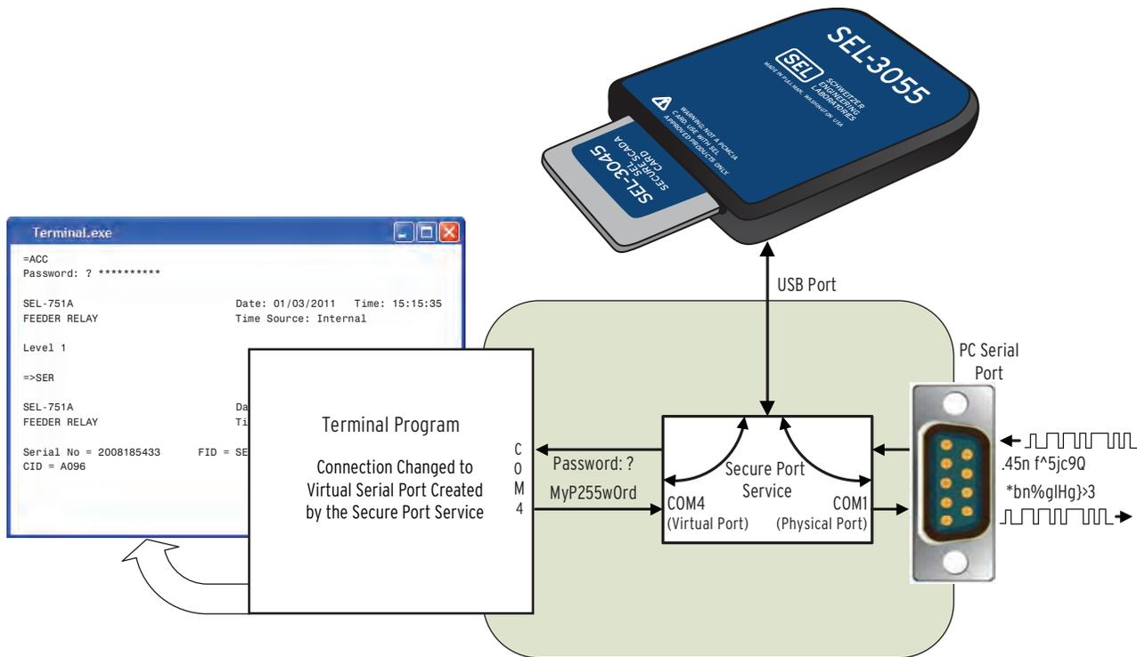
**Figure 1 Serial Data Encryption Using the PC Serial Security Kit**
