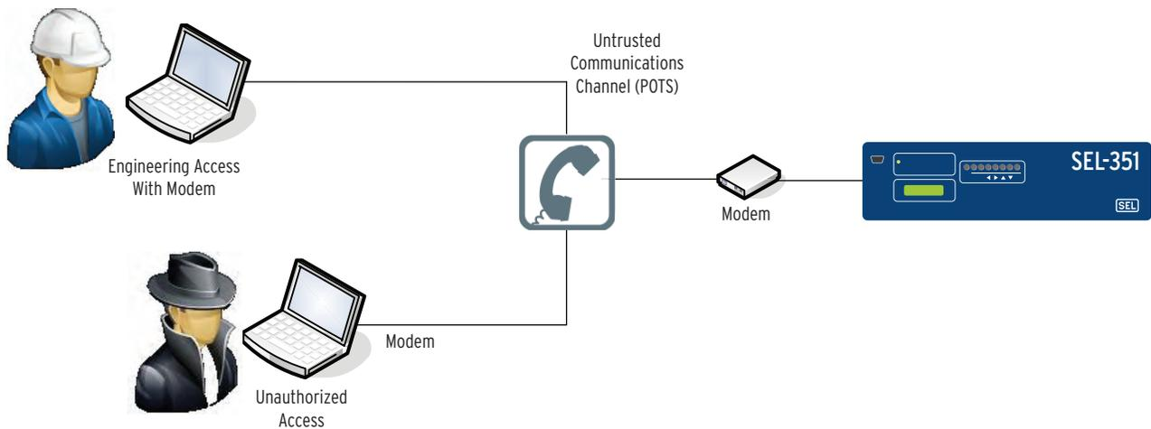
**Figure 2 Typical Engineering Access Communications Channel**
