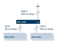
Time accuracy of  $\pm 40$  ns is maintained with cable delay compensation.
