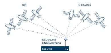
Satellite signal verification—the SEL-2488 and SEL-9524B GPS/GLONASS GNSS Antenna receive signals from two satellite constellations to validate GPS time signals, providing a layer of protection from GPS spoofing attacks.
