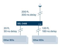
Time accuracy of  $\pm 40$  ns is maintained with cable delay compensation.
