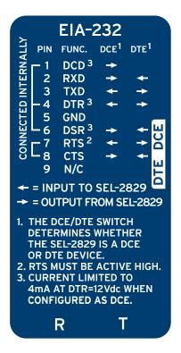
Label With EIA-232 Pin Usage Imprinted on the bottom of the device.
