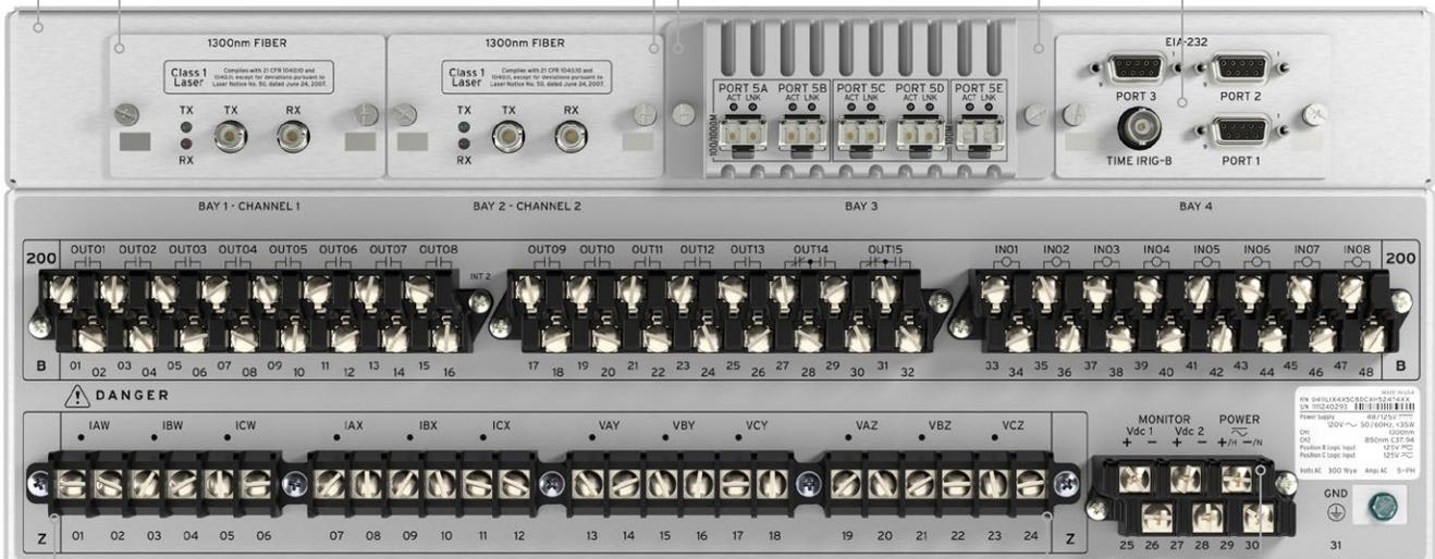
Six current and six voltage analog inputs support protection for substations with dual-breaker schemes.
