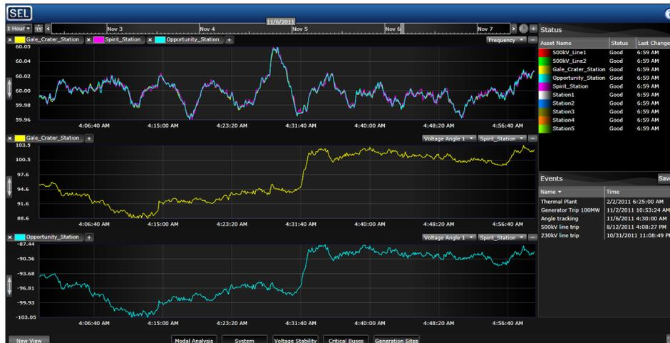
SEL-5078-2 SYNCHROWAVE Central Software provides visualization and analysis of power system operating conditions.
