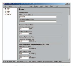
Develop settings using AcSELERATOR QuickSet® SEL-5030 Software.
