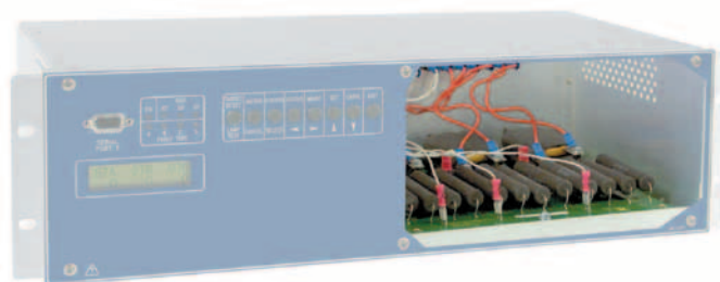
Cutaway view showing stabilizing resistors and MOVs.
