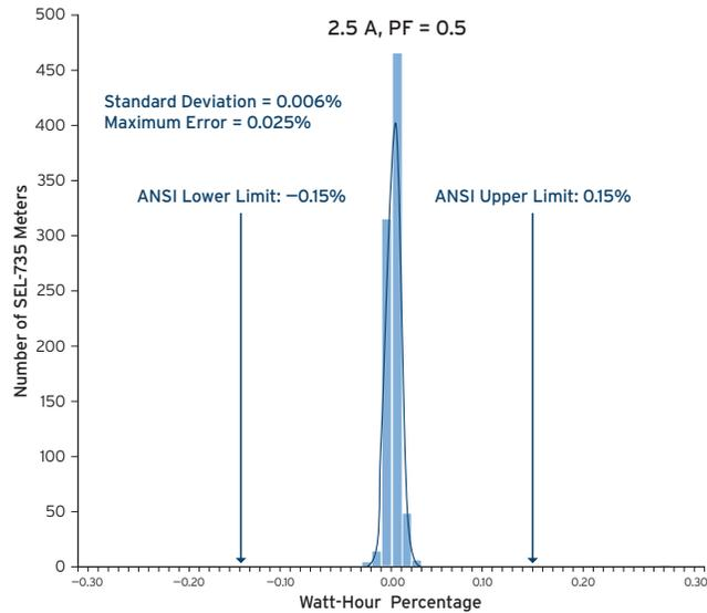
Accuracy-test results of approximately 1,000 SEL-735 Meters report a maximum error of 0.025 percent, outperforming ANSI 0.1 and IEC 0.1 S accuracy class requirements.
