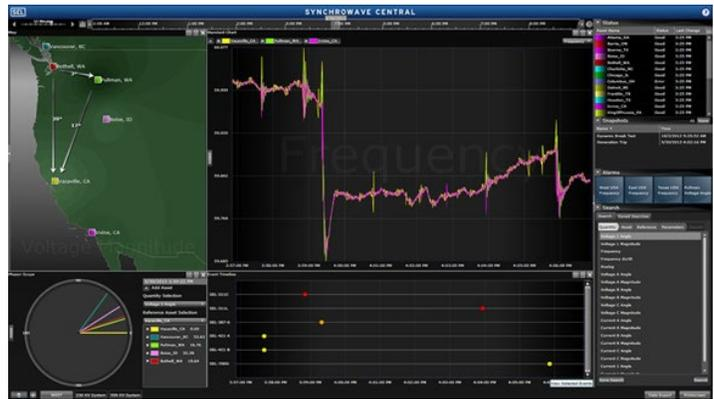
Monitor grid conditions with time-aligned synchrophasor messages.
