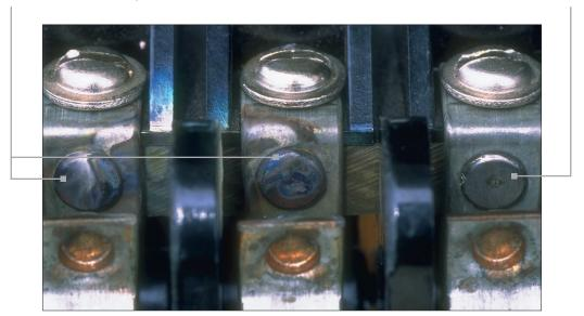
The single right contact was protected by the SEL-9501 under the same test conditions.
