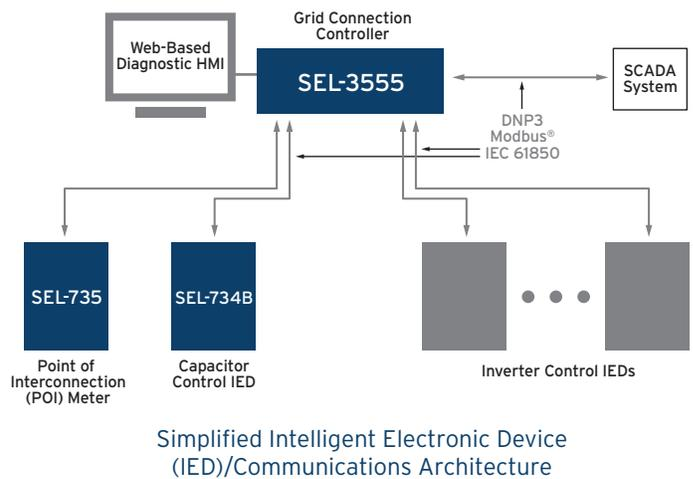
In addition to providing internal plant monitoring and control functions, the system also serves as a single-point interface with external systems, where it supplies plant data and accepts control commands from the area electric power system. This single-point interface simplifies the communications burden on the electric power system while providing the necessary functionality to maintain critical voltage support features for the bulk electrical system.
