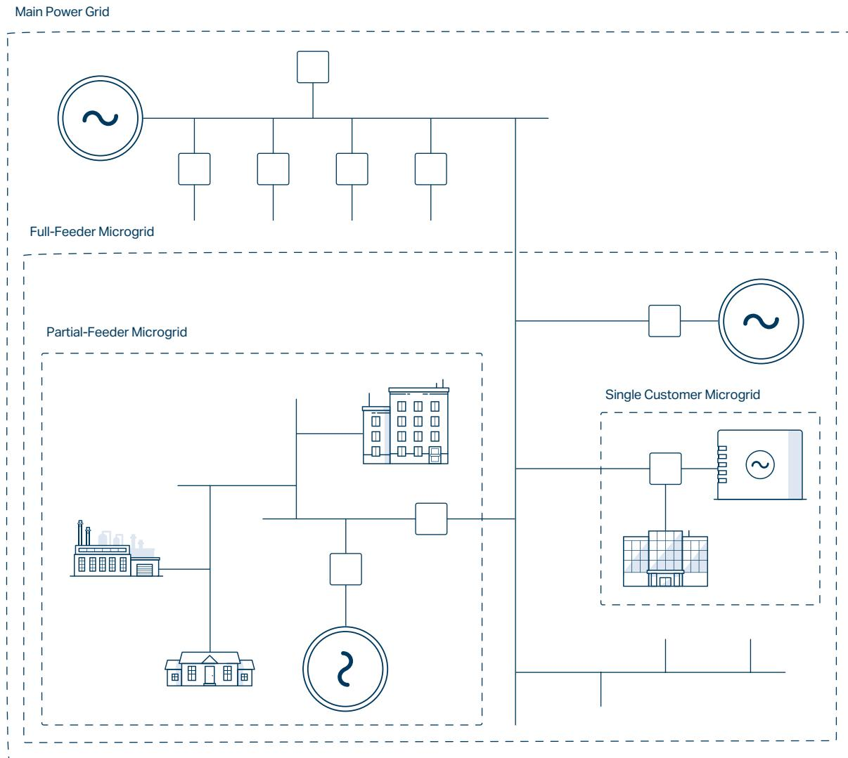
**Islanding Configuration Possibilities**—Within the microgrid, the SEL control allows one or more submicrogrids to operate, ensuring critical loads are always served.
