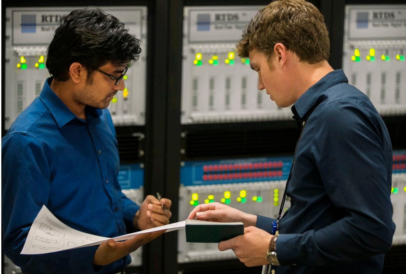
**Factory Acceptance Testing**—All microgrid control systems are thoroughly tested and configured before shipment using hardware-in-the-loop testing.
