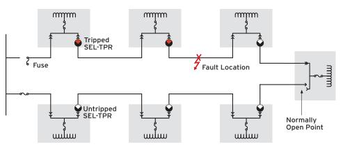
SEL-TPRs identify the faulted cable section within a loop of pad-mounted transformers that contain a normally open point.
