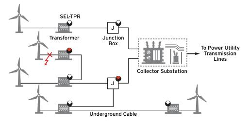
Three-phase wind farm circuit with SEL-TPRs indicating which string of turbines contains the fault.
