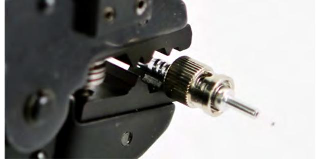
5. Slide the sleeve up to the base of the ST connector past the ribs on the barrel to ensure proper seating.
