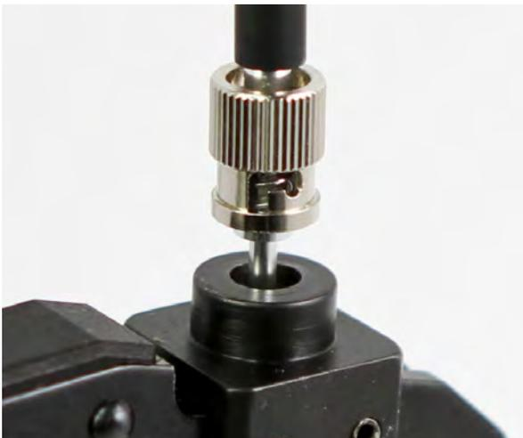
4. Slide the ST sleeve back far enough that the end of the ST connector can be placed in the jaws of the crimp tool without damaging the sleeve. Using the front hexagonal slot of the tool, crimp the end of the ST connector to the jacket of the fiber.
