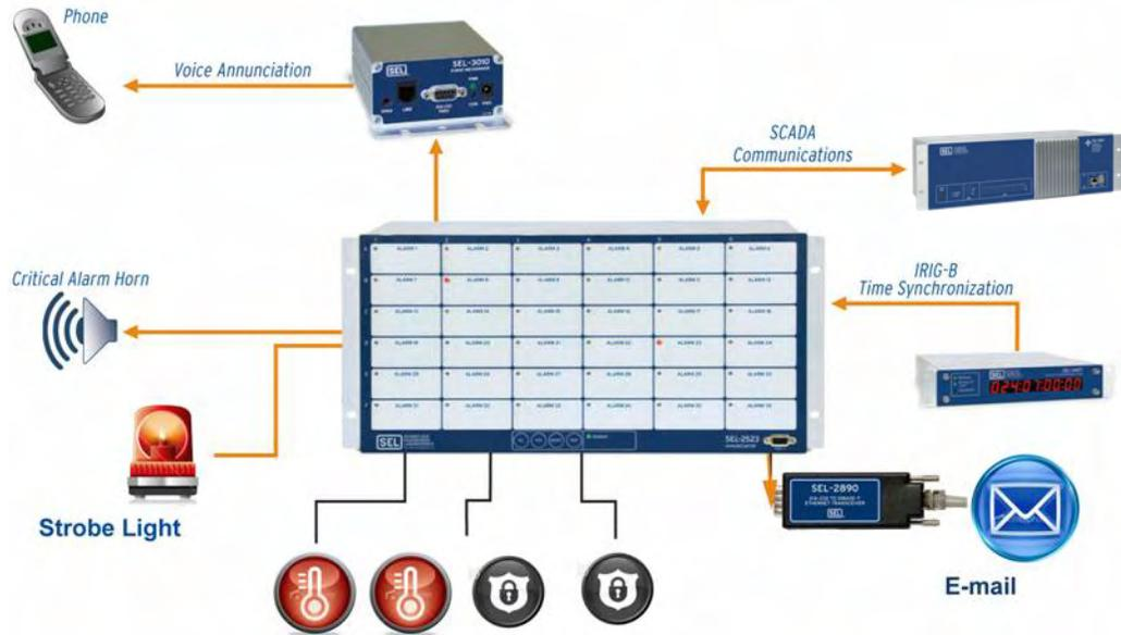
**Figure 2 Example security system alarm panel**
