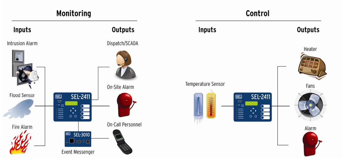
Figure 1 Building Monitoring and Control
