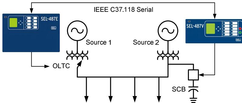
Figure 2 SEL-487E and SEL-487V Synchrophasor Real-Time Control
