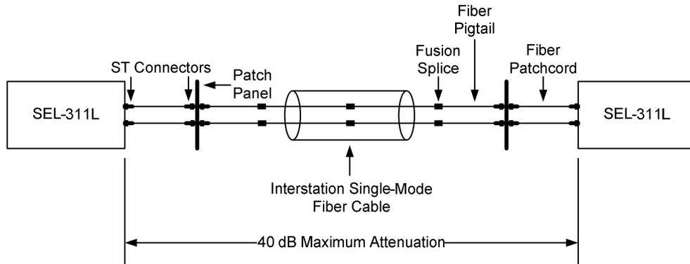
**Figure 1 Fiber System Loss Budget Example**
