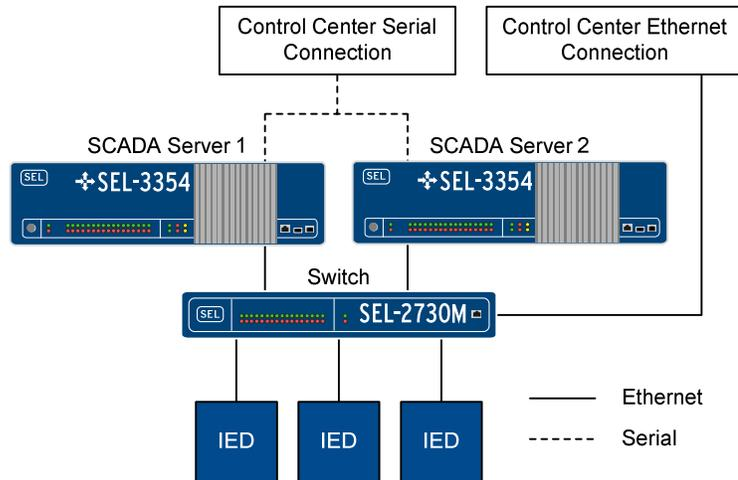
Figure 1 SCADA Server Based on SEL-3354 and Survalent SmartGateway Software
