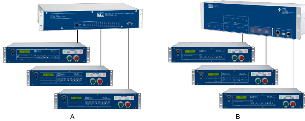
Figure 2 Communications Architecture Using (A) SEL-2100 or (B) SEL-3530 for Simultaneous Fault Clearing
