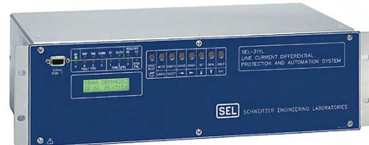
*Figure 2—The negative-sequence sensing elements in the SEL-311L introduce a new level of fault sensing and high-speed tripping. Standard features include programmable four-shot breaker auto-reclose with synchronism and voltage check logic for optimal system restoration.*
