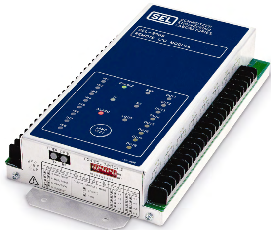
Figure 3—The flexibility of the SEL-2505 Remote I/O Module allows engineers to upgrade the design of the electrical system transfer-tripping scheme using a utility-grade device with improved reliability, compact design, and improved communications. Using MIRRORING BITS communications between devices, data are typically transferred at a rate of 11 ms. Another advantage is the ability to replace control wiring to outside cabinets with fiber-optic cable to reduce dc ground exposure.
