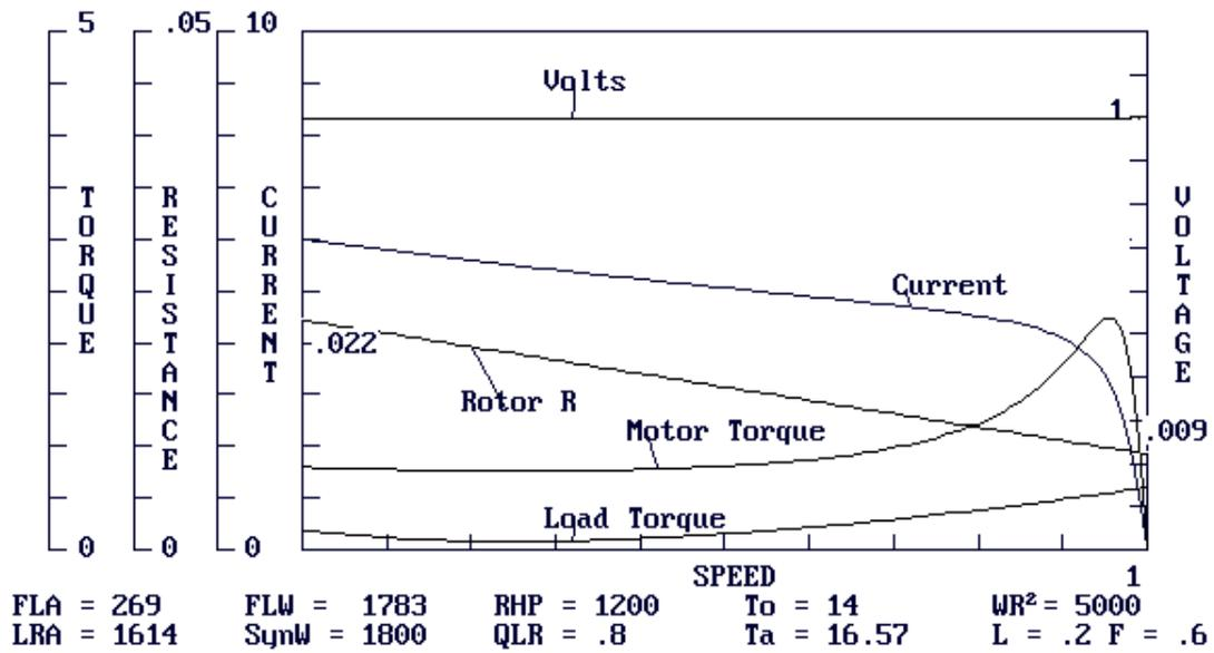
Figure 4: Current and Torque Versus Slip
