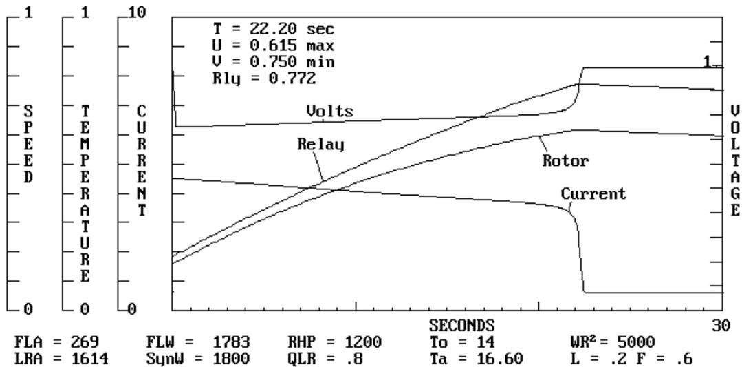
Figure 12: Plot of Motor Voltage, Current, and Rotor Hot Spot Temperature
