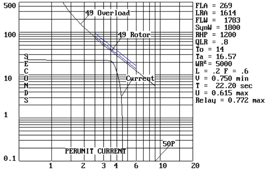
Figure 13: Log Plot of Current and SEL-501 Characteristic
