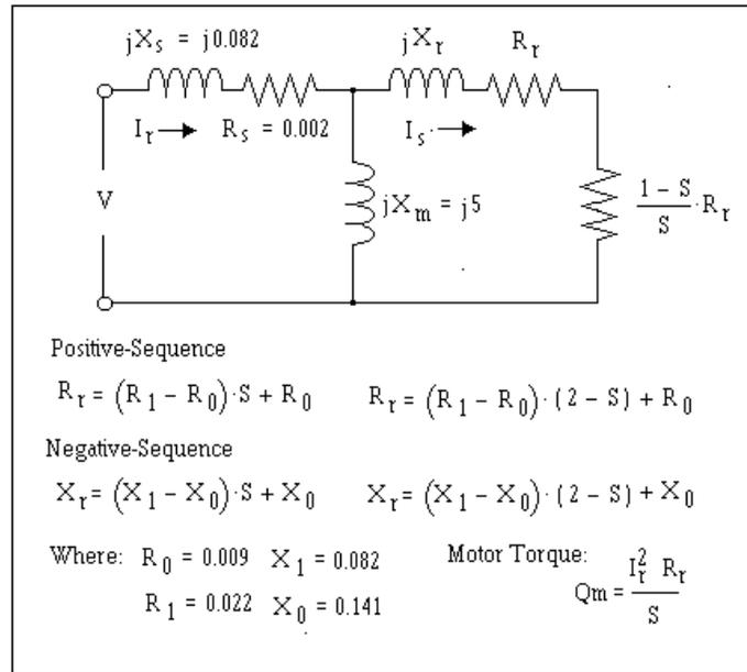
Figure 3: Motor Equivalent Circuit
