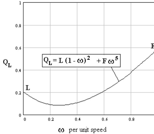
Figure 5: Contour of Load Torque
