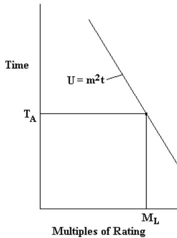
Figure 8: Time-Current Characteristic
