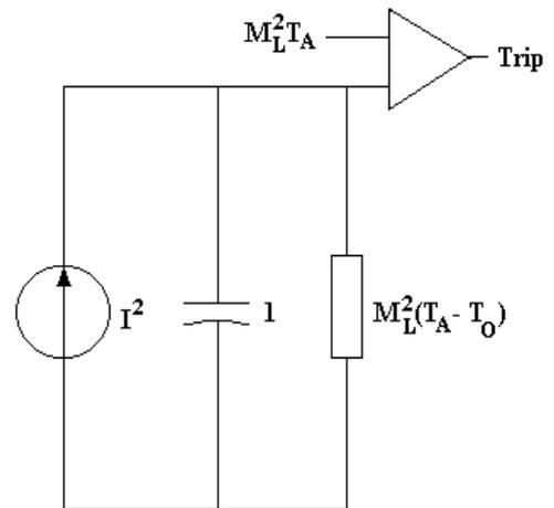
Figure 9: Electrical Analog With Thermal Resistance
