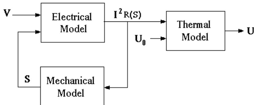
Figure 1: Motor Analysis Block Diagram
