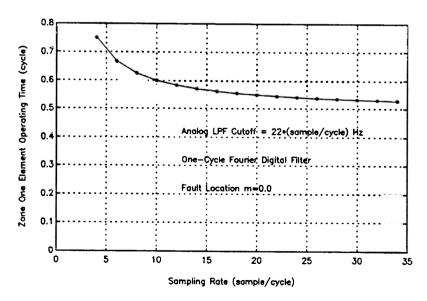
Figure 4.7 Operating Time vs Sampling Rate
