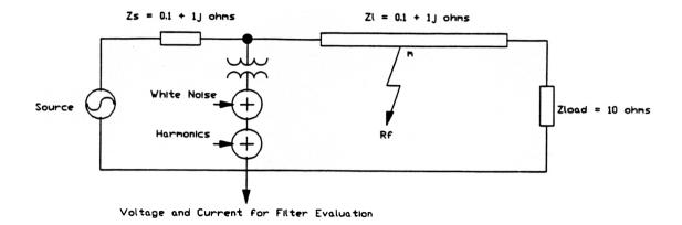
Figure 5.1 Power System Model
