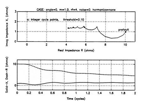
Figure 6.14 Kalman Filter with Threshold 0.10
