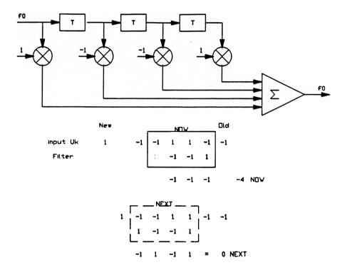
Figure 6.9 Convolution Filtering
