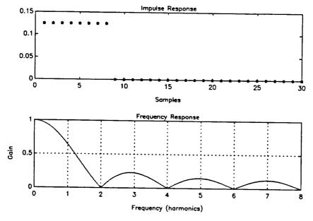
Figure 4.2 FIR Lowpass Filter  $y_k = [x_k + ... + x_{k-7}]/8$
