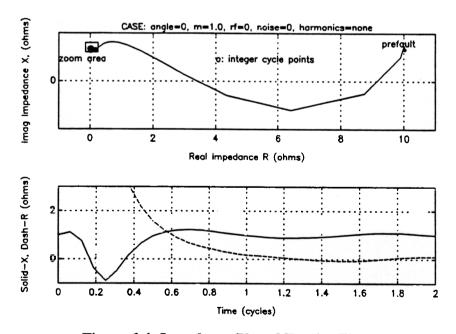
Figure 6.4 Impedance Plot of Fourier Filter
