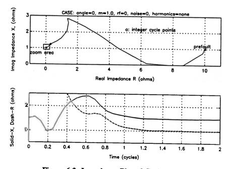
Figure 6.3 Impedance Plot of Cosine Filter
