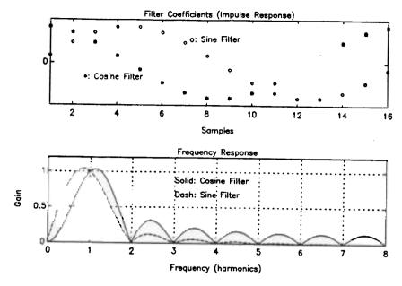
Figure 6.2 Cosine and Sine Filters
