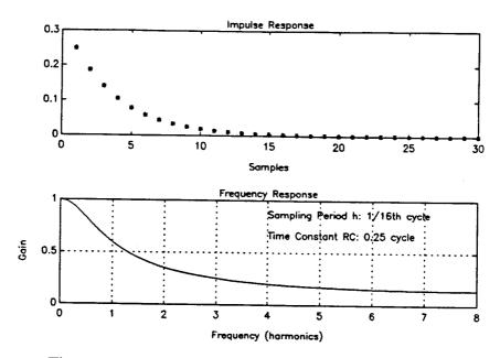
Figure 4.1 IIR Lowpass Filter  $y_k = (1/4)x_k + [1-(1/4)]y_{k-1}$
