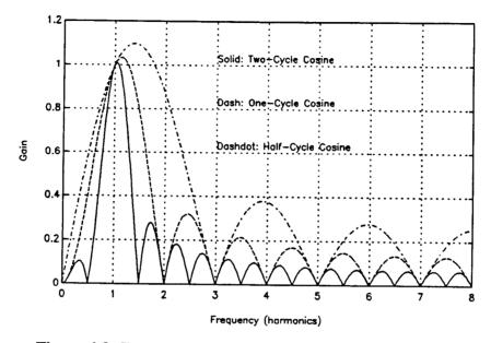
Figure 4.3 Frequency Responses of Half-, One- and Two-Cycle Window Cosine Filters
