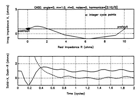
Figure 4.4 Impedance Plot of Half-Cycle Cosine Filter
