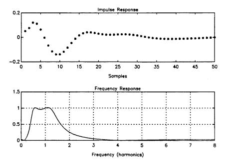
Figure 6.6 An IIR Bandpass Filter
