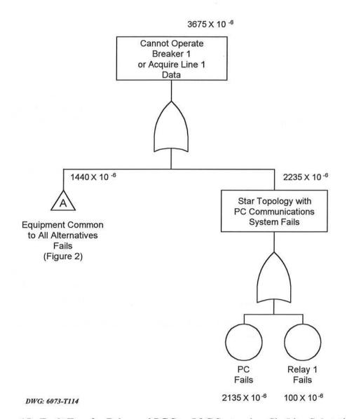
Figure 15: Fault Tree for Relay and PC Star I&C System in a Six-Line Substation
