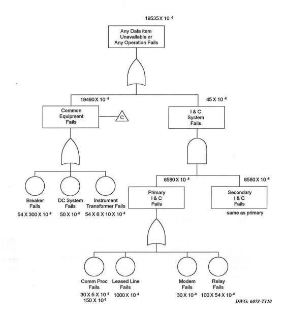
Figure 11: Fault Tree for Any Failure of Communications Processor I&C System for 54-Line Substation
