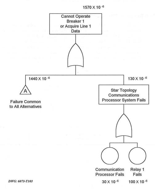
Figure 4: Fault Tree for Relay and Communications Processor Star I&C System in a Six-Line Substation
