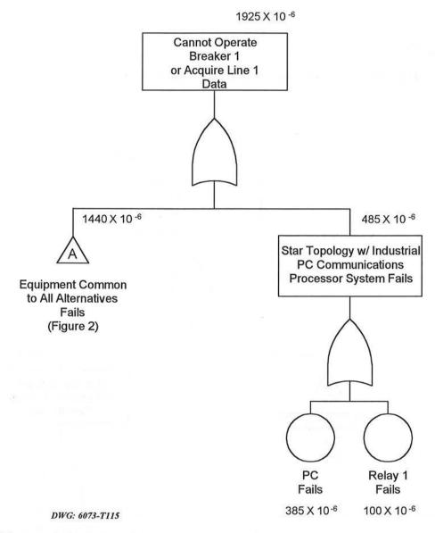
Figure 16: Fault Tree for Relay and Industrial PC Star I&C System in a Six-Line Substation
