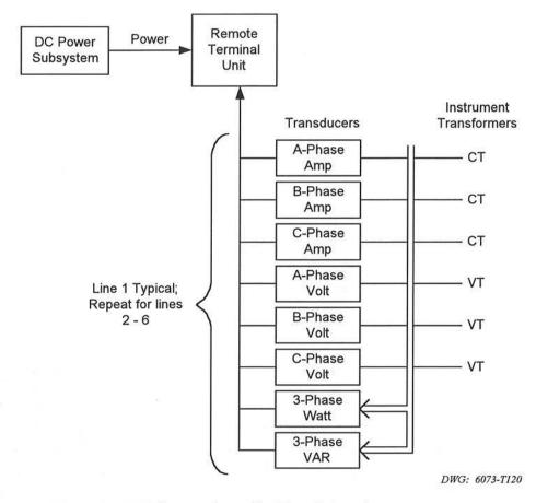
Figure 1: Example RTU System for a Six-Line Substation
