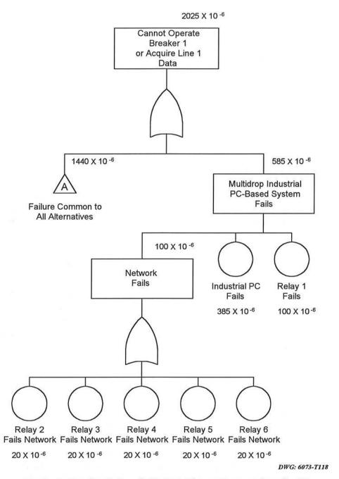
Figure 17: Fault Tree for Industrial PC Multidrop Network in a Six-Line Substation
