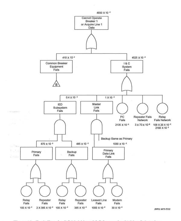
Figure 13: Fault Tree for PC Multidrop I&C System for 54-Line Substation
