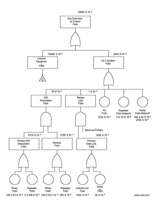
Figure 14: Fault Tree for Any Failure of PC Multidrop I&C System for 54-Line Substation
