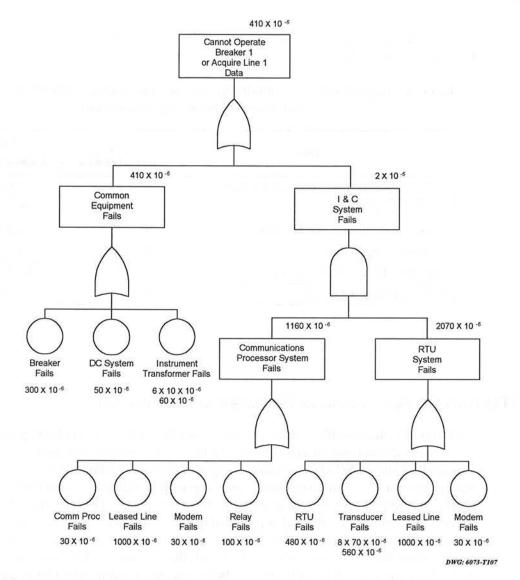
Figure 8: Fault Tree for RTU and Communications Processor/Relay System in a Six-Line Substation
