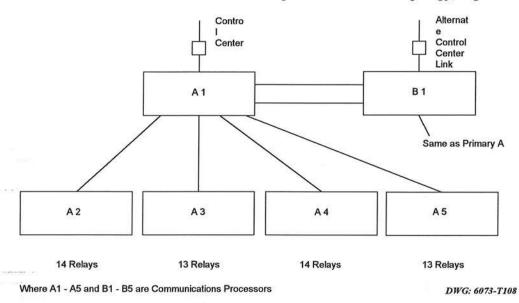
Figure 9: Block Diagram of Communications Processor I&C System for 54-Line Substation
