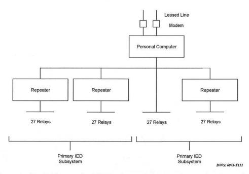
Figure 12: Block Diagram for PC Multidrop I&C System for 54-Line Substation
