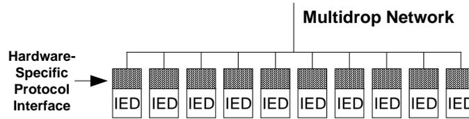
Figure 5: Multidrop Network IED Interface
