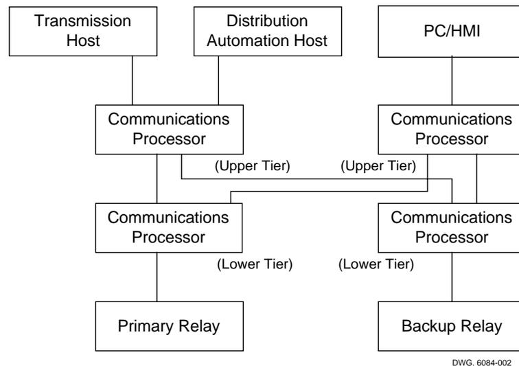
**Figure 9: SI System Two-Tier Architecture**
