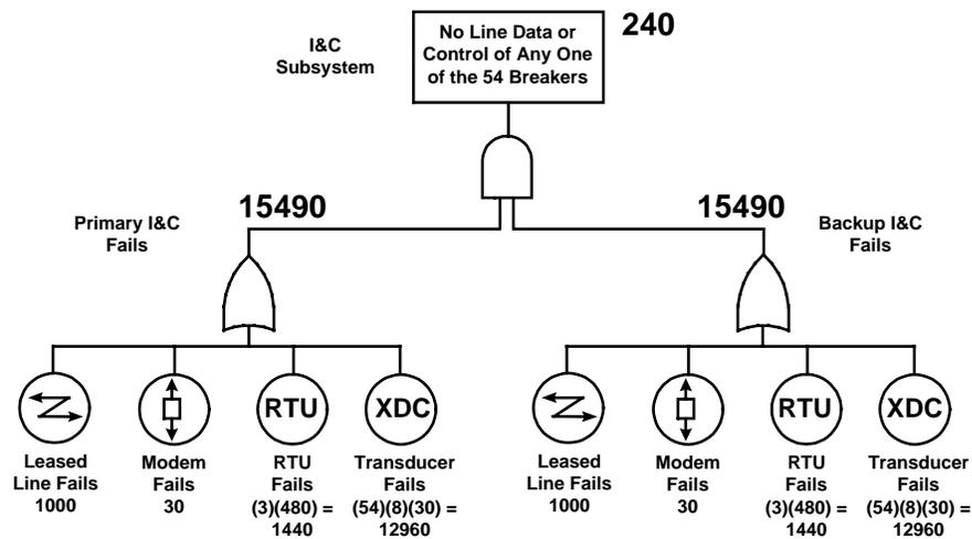
**Figure 3: Fault Tree for RTU Centric Westmoreland I&C System**
