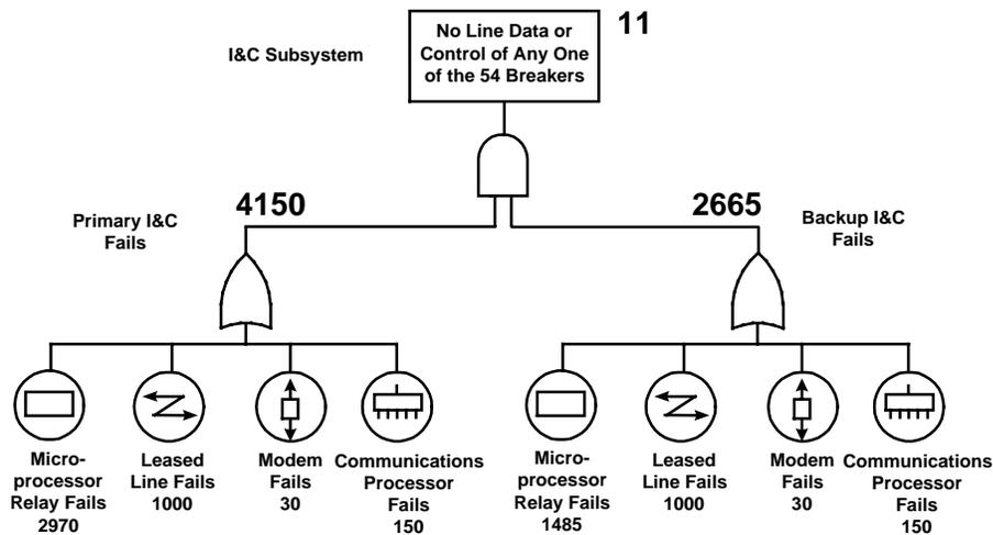
**Figure 8: Communications Processor Star Relay Network Centric Westmoreland I&C System**
