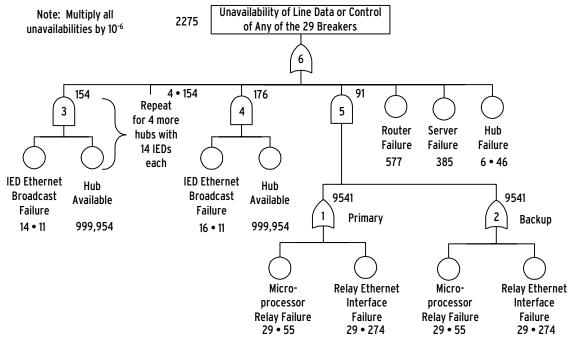
Figure 2: Shared Hub Fault Tree
