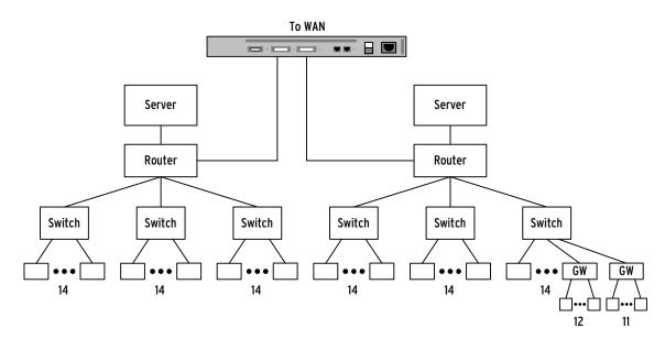
Figure 6: Redundant Servers, Routers, and Switches LAN Block Diagram
