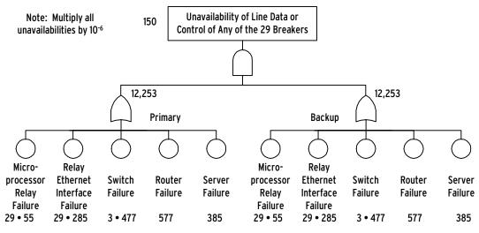
Figure 7: Redundant Servers, Routers, and Switches Fault Tree
