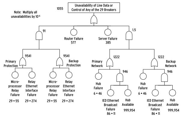
Figure 5: Redundant Shared Hub Fault Tree
