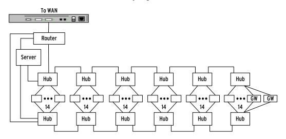
Figure 4: Redundant Shared Hub Block Diagram
