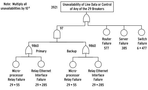
Figure 3: Switch Fault Tree
