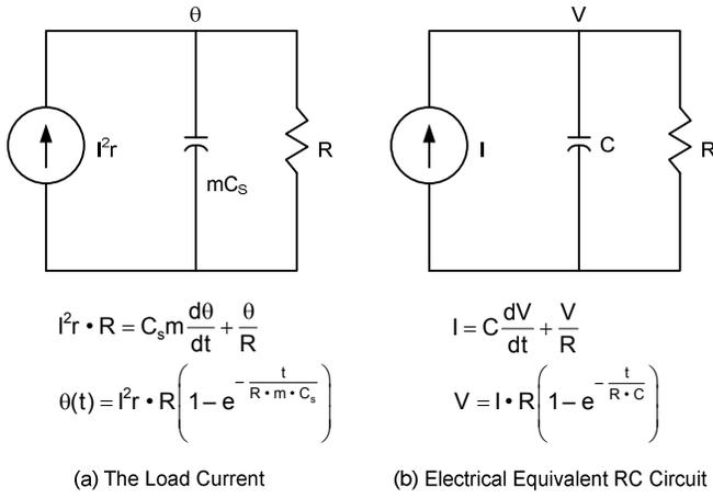
Fig. A2. Equivalence Between a Thermal System and a Parallel RC Circuit
