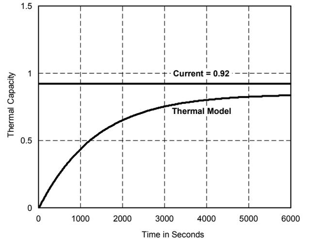
Fig. 2. Response of Models to a Current Less Than the Service Factor ( $I = 0.92$ )
