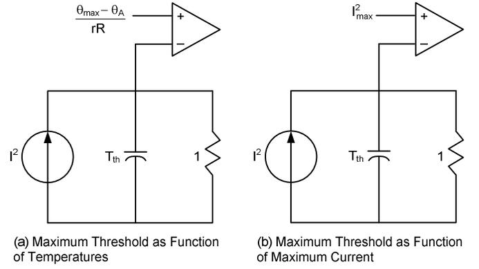
Fig. A3. Electrical RC Equivalent of Thermal Process
