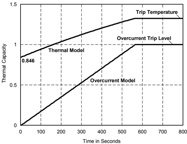
Fig. 4. Thermal and Overcurrent Model Response With Initial Temperature = 0.846
