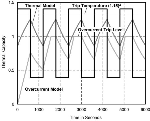
Fig. 3. Response of the Models to a Cyclic Overload Current
