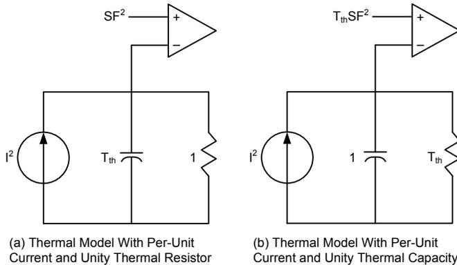
Fig. A4. Electrical RC Equivalent of Thermal Process
