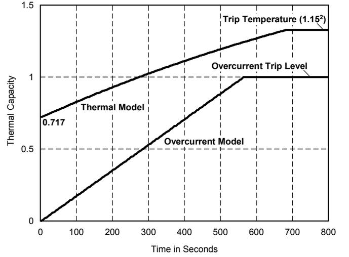
Fig. 5. Thermal and Overcurrent Model Response With Initial Temperature = 0.717
