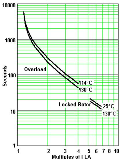
Fig. 1. Hot and Cold Limit Curves for a 400-Horsepower Motor, SF = 1.15
