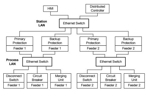
Figure 2 Station LAN and Multiple-Segment Process LAN Design
