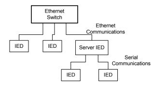
Figure 6 Hybrid Ethernet and Serial LAN
