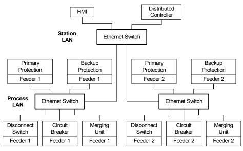
Figure 3 Merged Station and Process LAN Design
