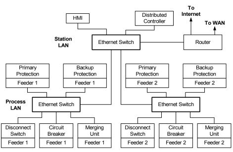
Figure 4 External Connections to Substation Communication Network
