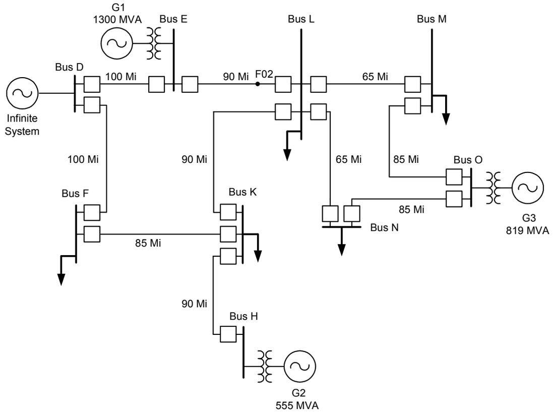
Figure 22 Multimachine System Used in Example 1
