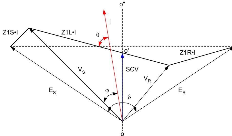
**Figure 4** Voltage Phasor Diagram of the Two-Source System
