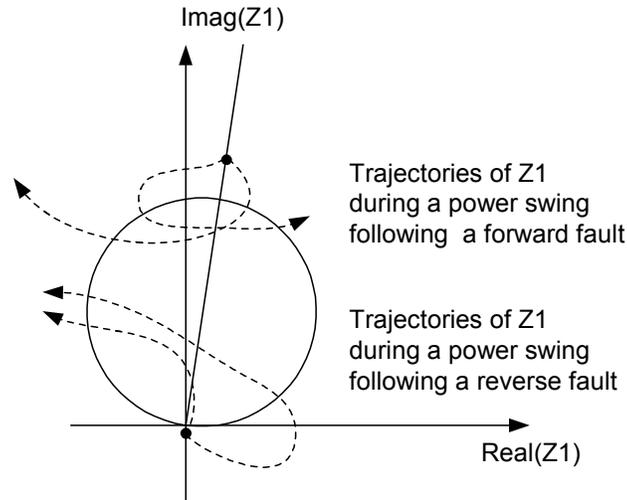
**Figure 12** Type of Faults Detected by the DPSB Function
