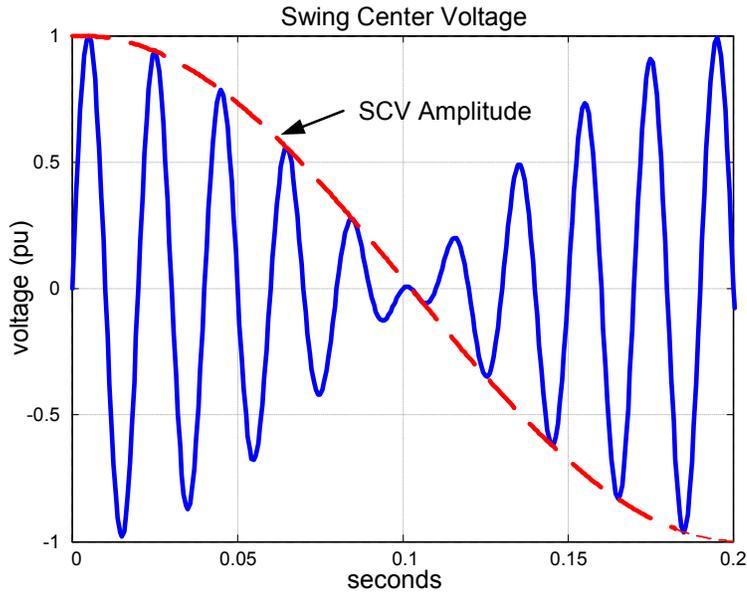
**Figure 5** Swing-Center Voltage During an OOS Condition
