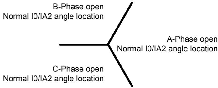
**Figure 18** I0/IA2 Angle Supervision During Pole-Open Situation
