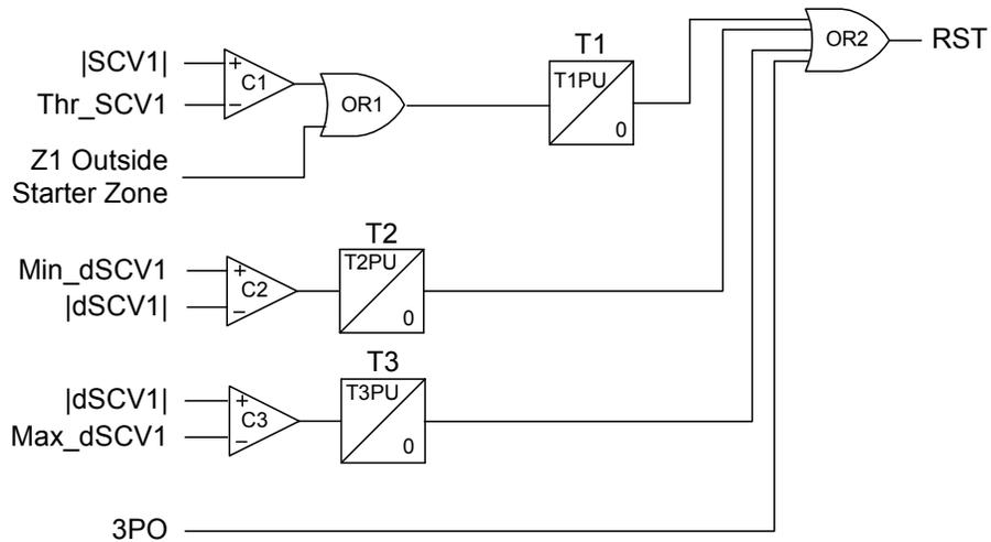
**Figure 14** Reset Logic
