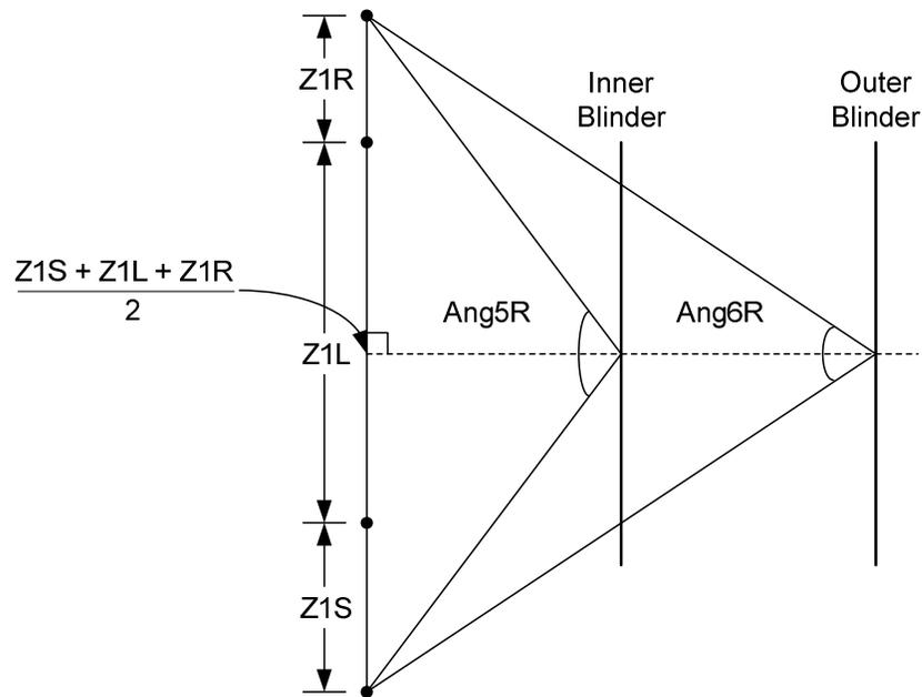
**Figure 3** Equivalent Two-Source Machine Angles During OOS
