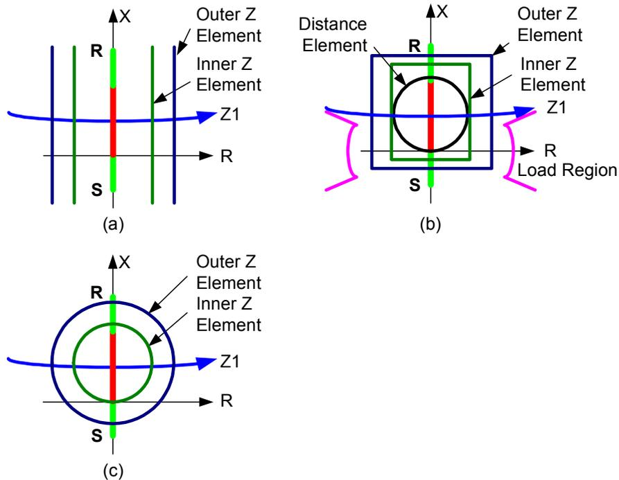
**Figure 1** Conventional Blinder Schemes for Power-Swing Detection
