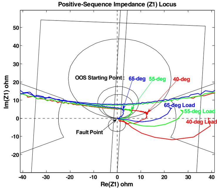
**Figure 27** Impedance Trajectories of Example 2 With Different Loads
