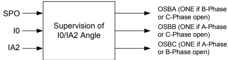
**Figure 19** Fault-Detector Logic During a Pole-Open Situation
