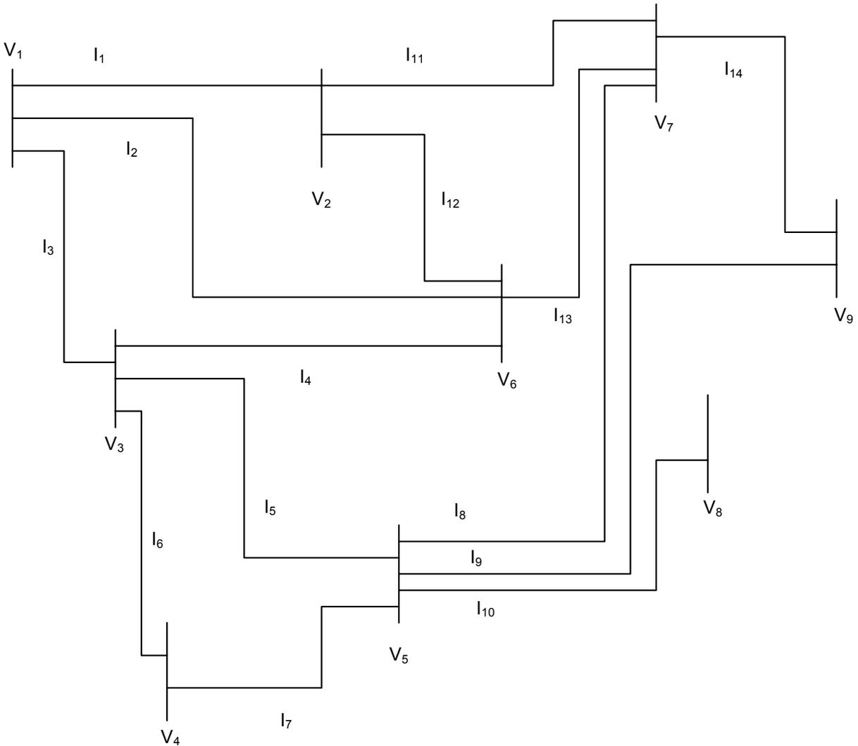
**Figure 4** Example System for State Measurement Requirements
