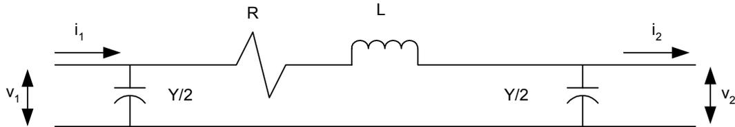
**Figure 2** Simple Model of a Transmission Line
