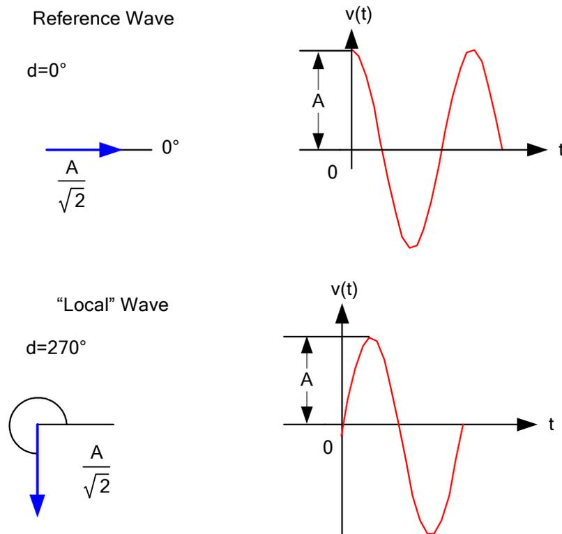
**Figure 1** Reference Wave and "Local" Wave With Angular Comparison
