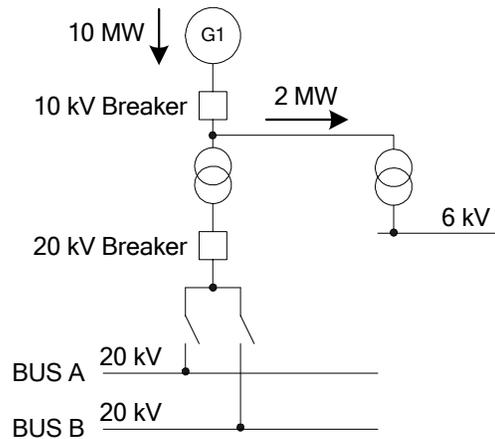
Fig. 6. Generator with tapped load
