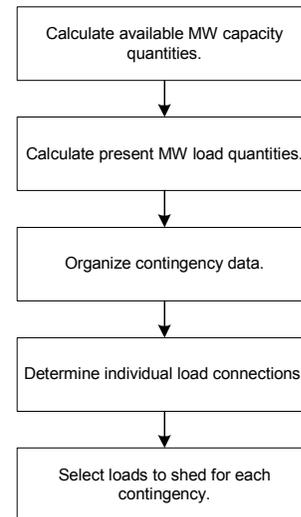
Fig. 8. Basic load selection algorithm
