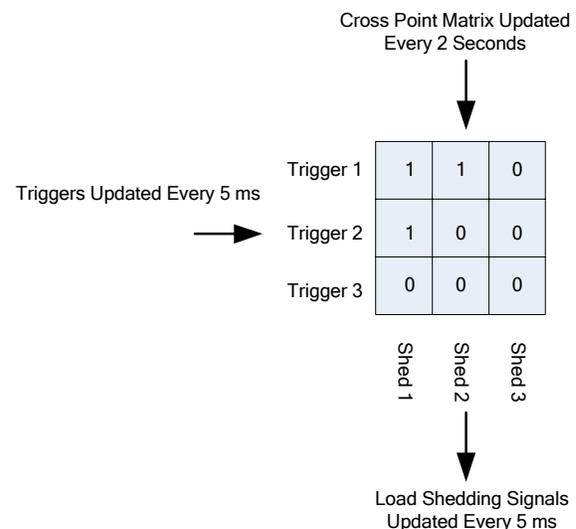
Fig. 15. Example 3x3 Cross Point Switch Matrix
