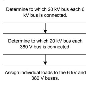
Fig. 12. Determine individual load connections
