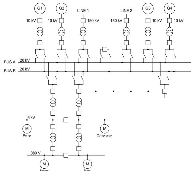
Fig. 1. Simplified one-line diagram of plant power system
