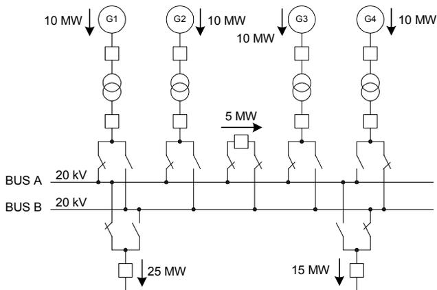
Fig. 7. 20 kV tie breaker trip (Bus B overloaded) contingency
