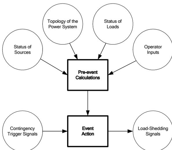
Fig. 2. Conceptual architecture of the load shed system
