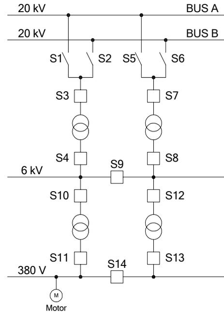
Fig. 13. Connection of a load to the 20 kV bus
