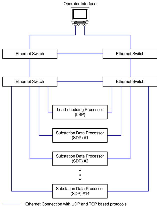
Fig. 5. Physical architecture between substations
