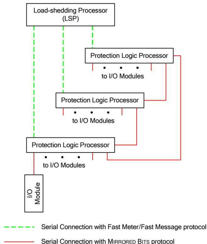
Fig. 3. Physical architecture of the load-shedding system
