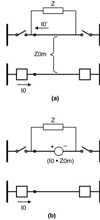
Fig. 5. Simple Ways to Visualize the Zero-Sequence Mutual Coupling in Parallel Lines
