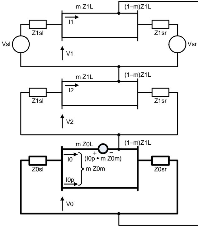
Fig. 6. Phase-to-Ground Fault in One of Two Parallel Lines With Zero-Sequence Mutual coupling
