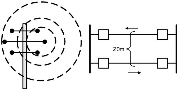
Fig. 4. Flux Linkage From One Line to the Other
