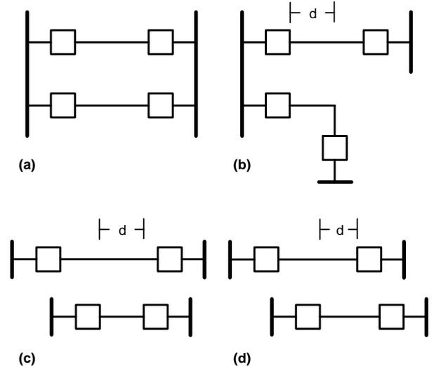
Fig. 1. Possible Configurations of Parallel Lines in Power Systems
