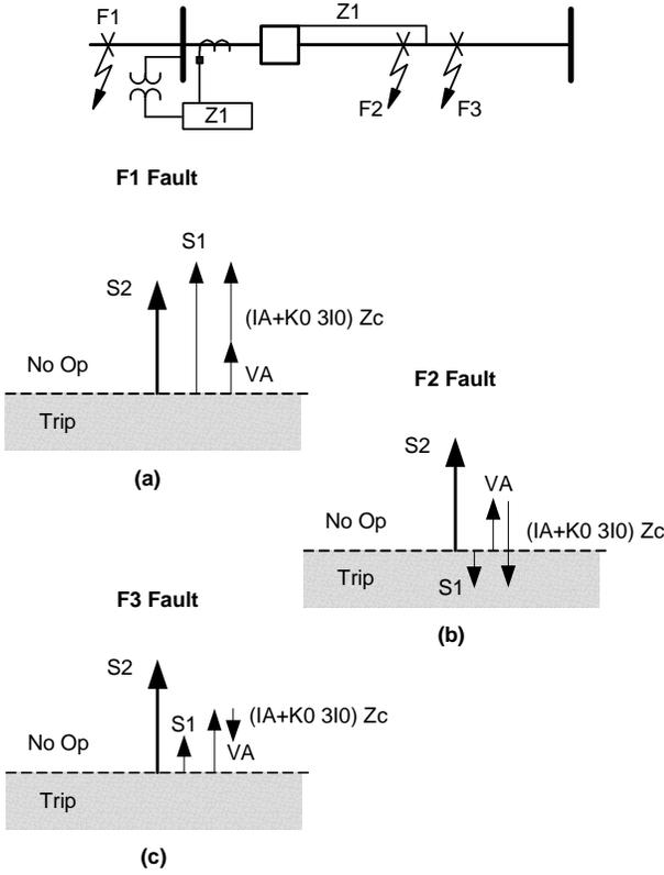
Fig. 9. Distance Relay Operation
