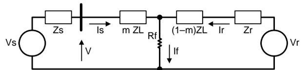
Fig. 7. Single-Phase Development of the Takagi Algorithm
