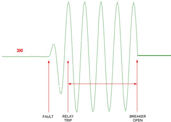
Fig. 17. Filtered 3I0 and Fault Clearing Sequence
