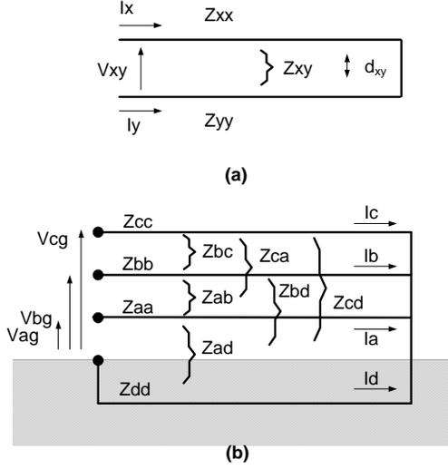
Fig. 2. (a) Two-Conductor Model (b) Three-Phase System With "Equivalent" Ground Conductor
