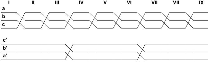
Fig. 3. Totally Transposed Parallel Lines
