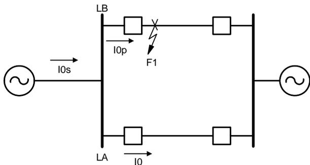
Fig. 15. Strong Source, Parallel Line Ground Fault Effect on the Healthy Line-Relay
