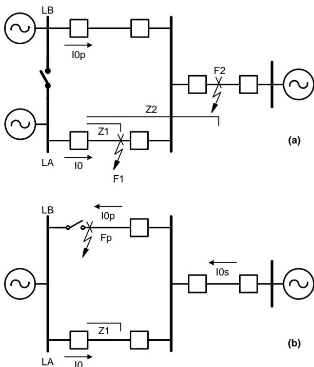
Fig. 13. Parallel Lines With a Single Common Bus
