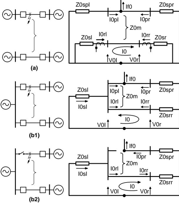
Fig. 8. Wrong Directional Determinations for Ground Directional Relays
