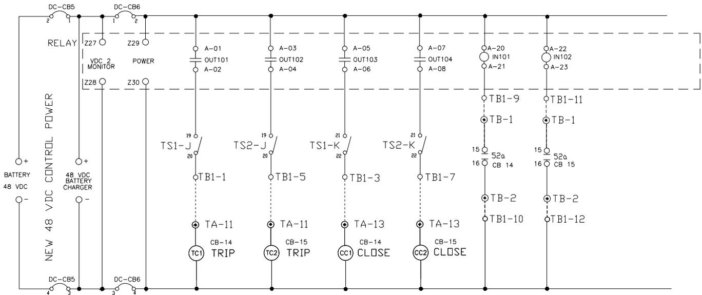
Fig. 9. DC Breaker Control Schematic
