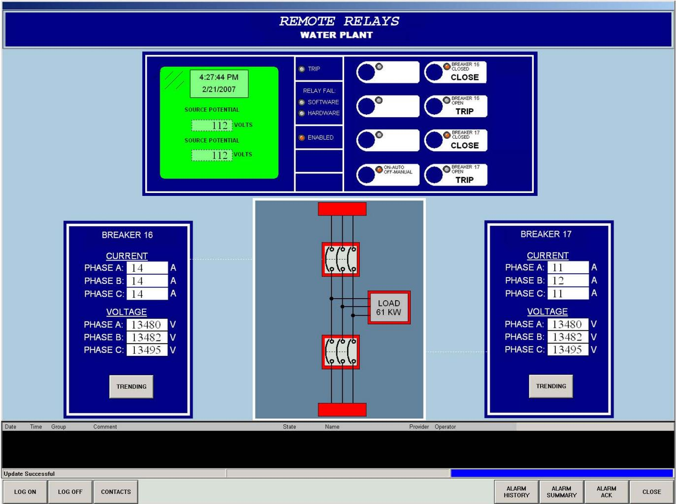
Fig. 16. Example SCADA HMI Screen
