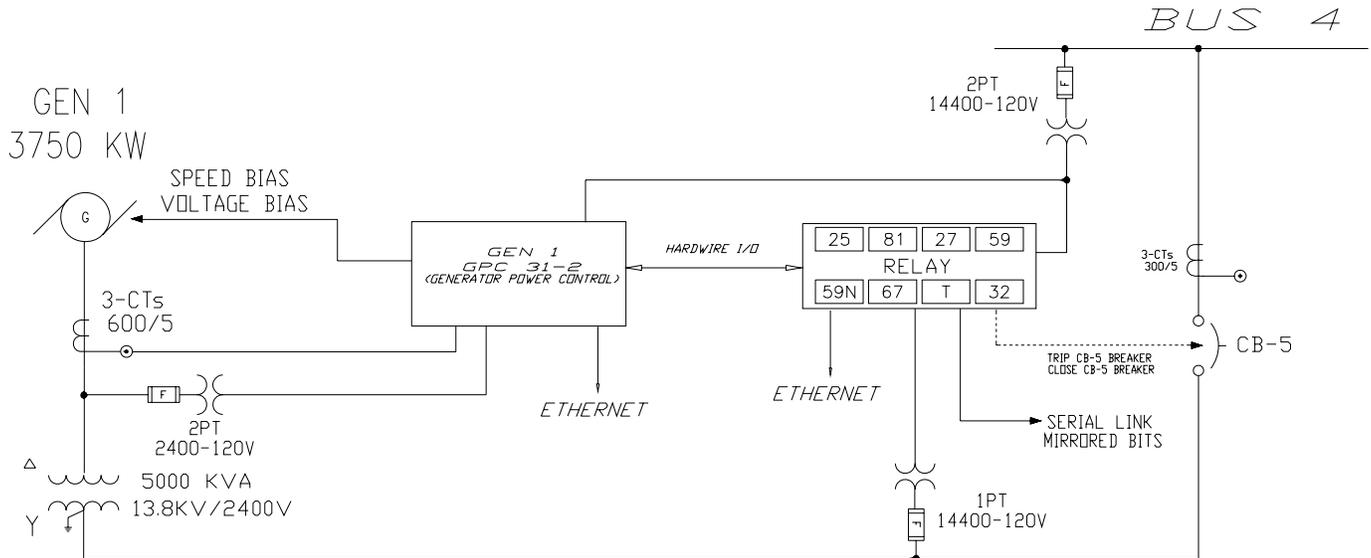
Fig. 14. Hardware Interconnections for Generator Controls
