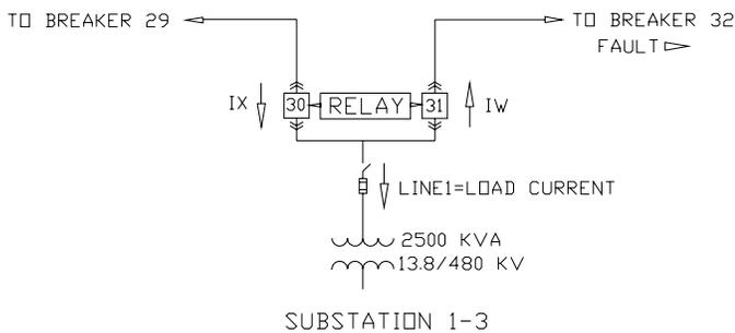
Fig. 6. Fault on Line Protected by Breaker 31
