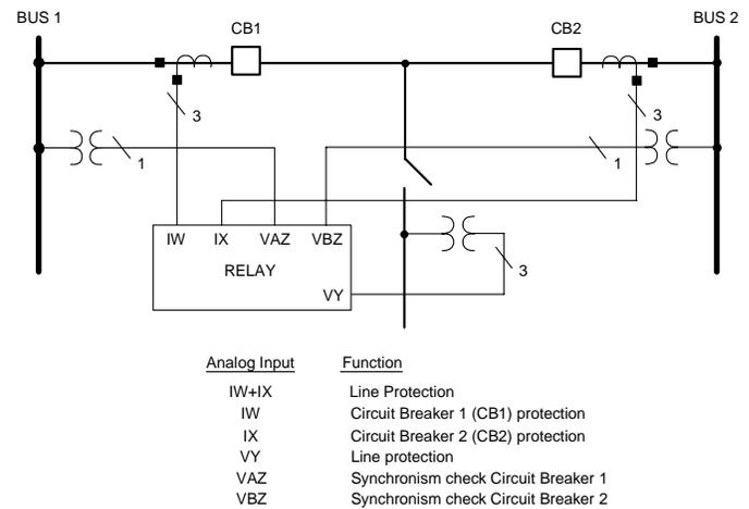
Fig. 3. Example of a Relay Configuration Provided by the Manufacturer
