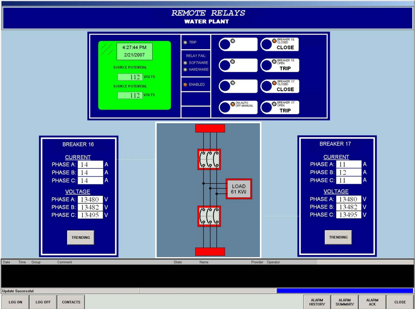
Fig. 16. Example SCADA HMI Screen
