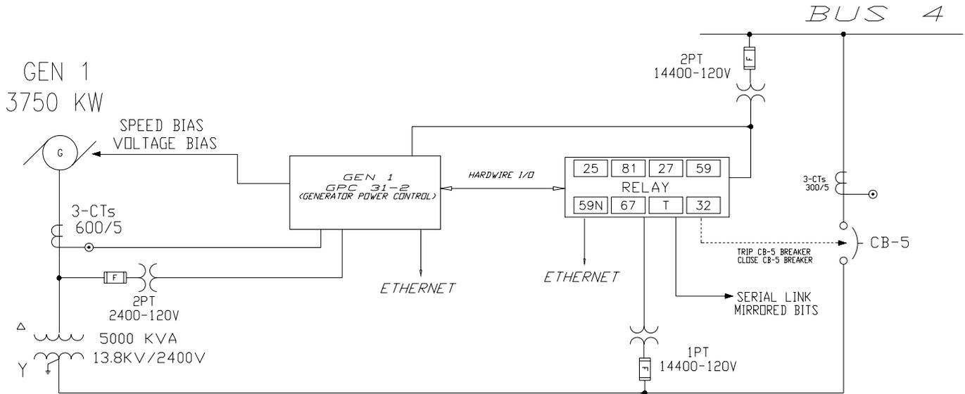
Fig. 14. Hardware Interconnections for Generator Controls
