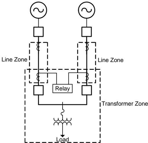
Fig. 2. Relay Protection Zones for Remote Substations
