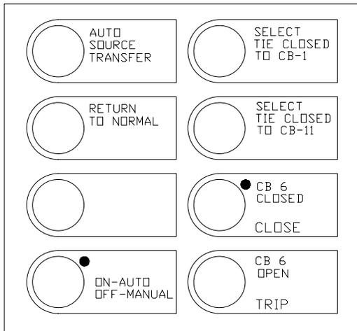
Fig. 12. Automatic Transfer Pushbuttons
