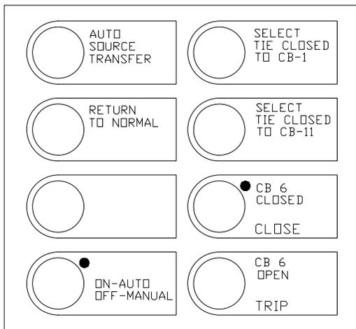
Fig. 12. Automatic Transfer Pushbuttons
