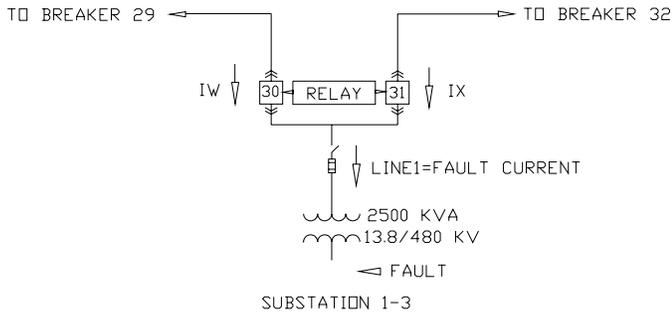
Fig. 4. Fault on Remote Station Bus or Transformer
