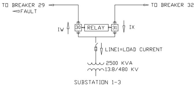
Fig. 5. Fault on Line Protected by Breaker 30
