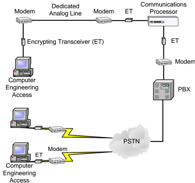
Fig. 5. Adding Serial Encrypting Transceivers Provides Data Security
