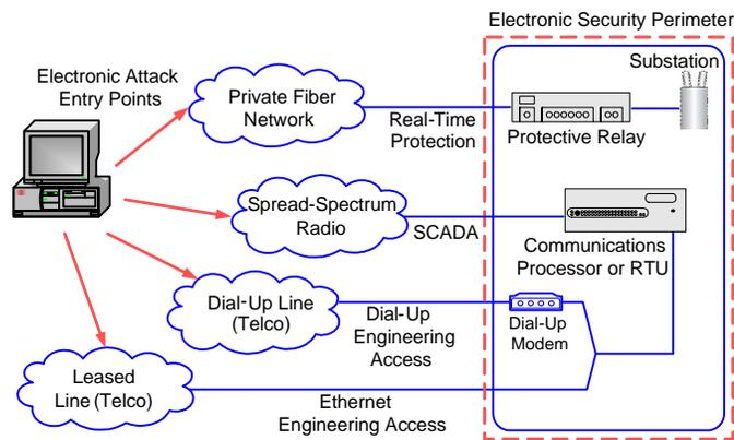
Fig. 2. Typical Modern Substation Network
