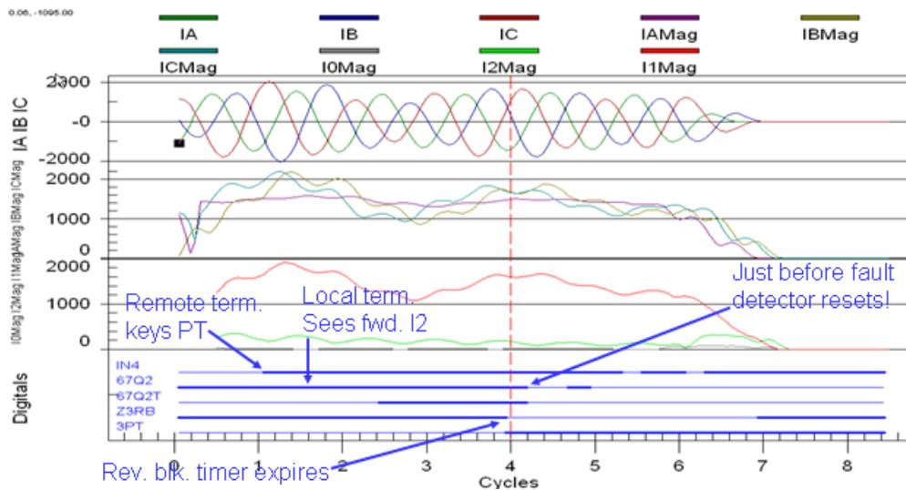
Fig. 12. 5L13 relay at WSN during misoperation
