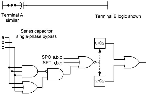
Fig. 8. Series capacitor bypass logic
