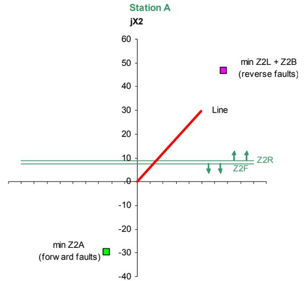
Fig. 1. Typical directional element settings
