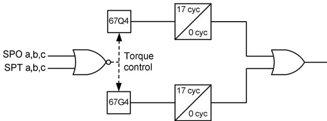
Fig. 9. Sensitive logic with long time delay
