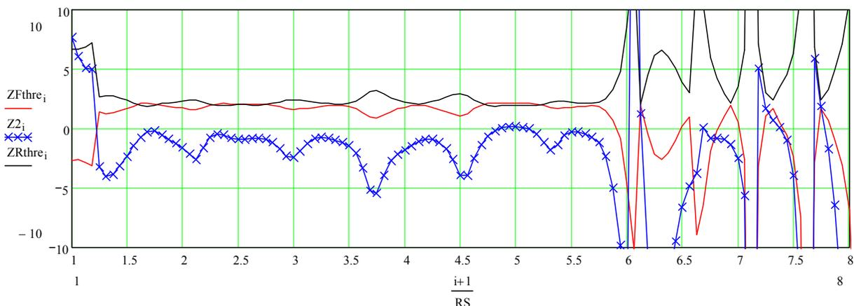
Fig. 13. Negative-sequence impedance element during subharmonic current flow on B- and C-phases
