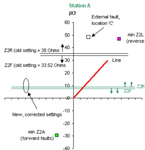
Fig. 4. External fault based on fault study
