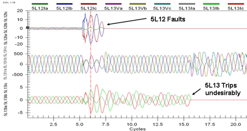
Fig. 11. Disturbance records of line current and bus voltage during fault
