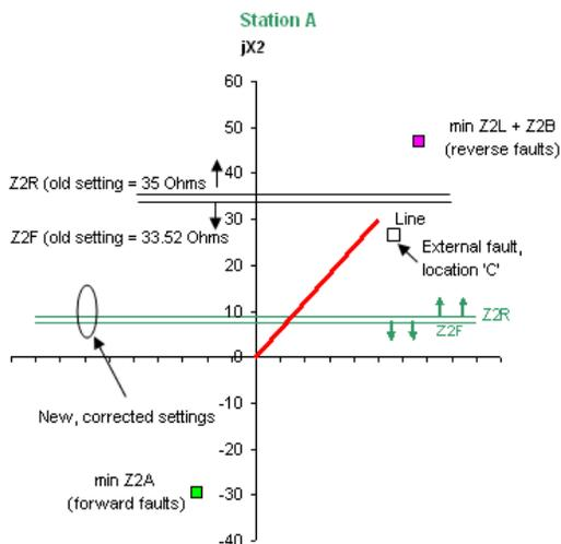
Fig. 3. Terminal A sees forward for external fault
