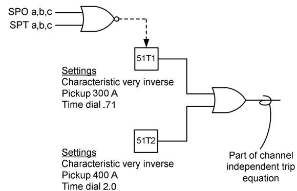
Fig. 7. Open-pole 51T1 and 51T2 application
