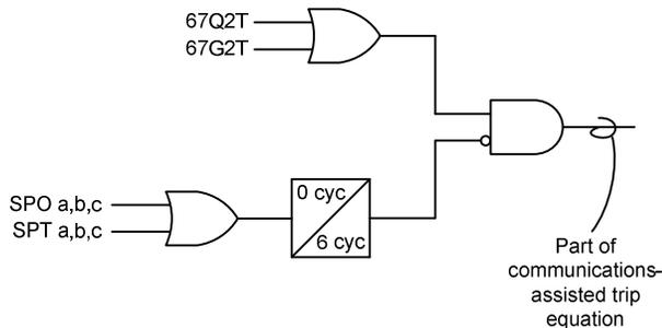
Fig. 5. Disable elements during open pole
