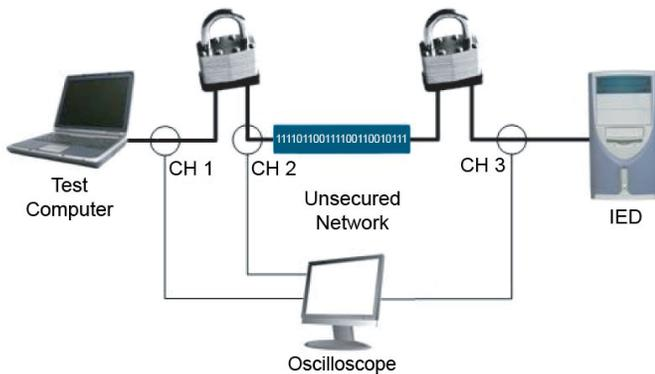
Fig. 7. Test Configuration
