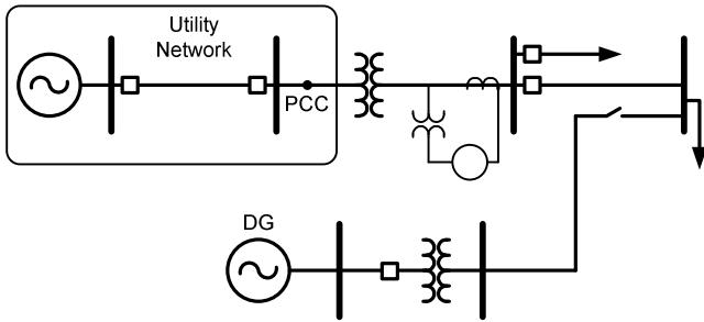
Fig. 1. DG interconnection with a utility network
