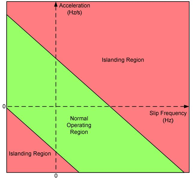
Fig. 3. Islanding detection characteristic using wide-area measurements
