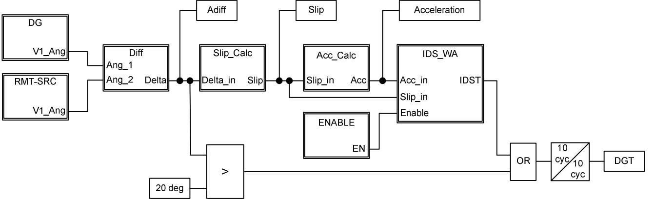
Fig. 4. Islanding detection logic based on local and remote time-synchronized measurements
