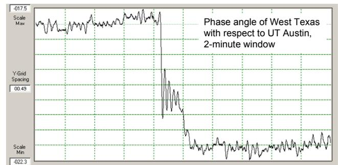
Fig. 17. Voltage phase angle response to generator trip
