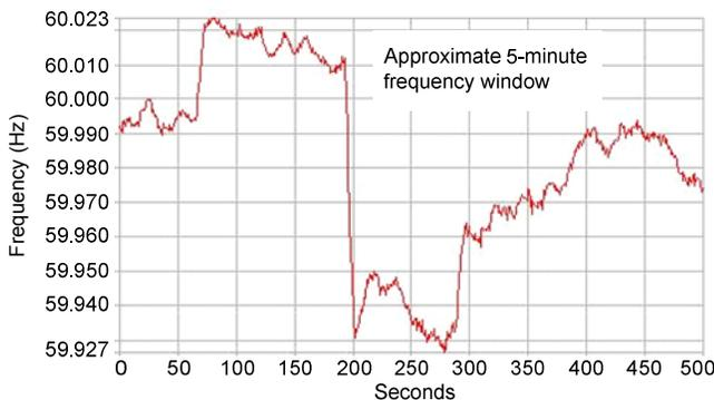
Fig. 14. Frequency excursion due to generator trip on March 6, 2009
