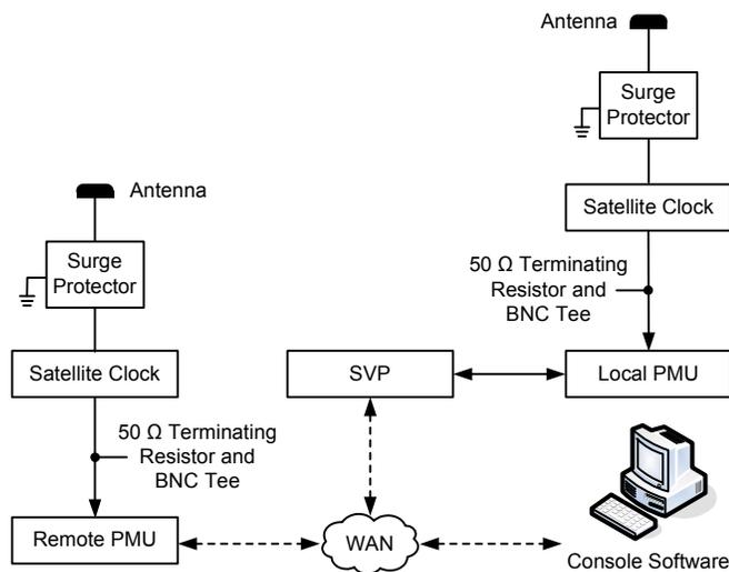
Fig. 4. Block diagram of system equipment setup
