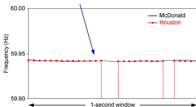
Fig. 39. One-second zoom-in shows 3 dropouts out of 30 points
