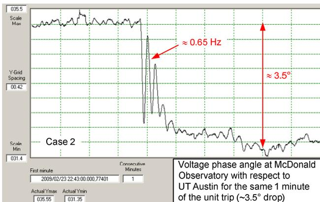
Fig. 10. Voltage phase angle change during generator trip
