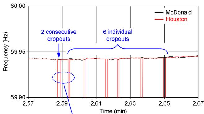
Fig. 38. Six-second zoom-in of the Houston dropout cluster
