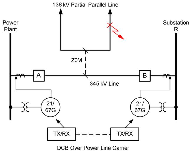
Fig. 17. 345 kV line with 138 kV line underbuild
