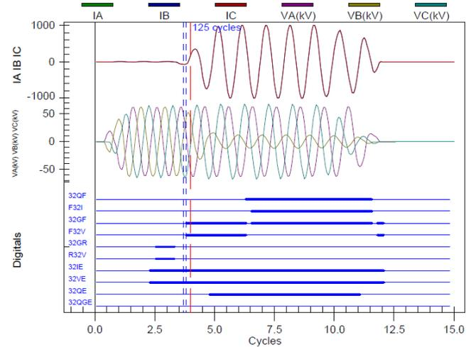
Fig. 12. Automatic switching ground directional element response
