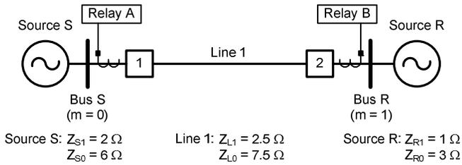
Fig. 6. Example system to evaluate directional element performance
