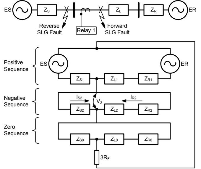
Fig. 4. Symmetrical component diagram for single-line-to-ground (SLG) faults
