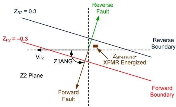
Fig. 15. A negative  $Z_{F2}$  setting increases security
