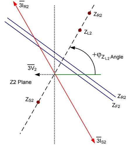
Fig. 5. Measured negative-sequence impedance yields fault direction
