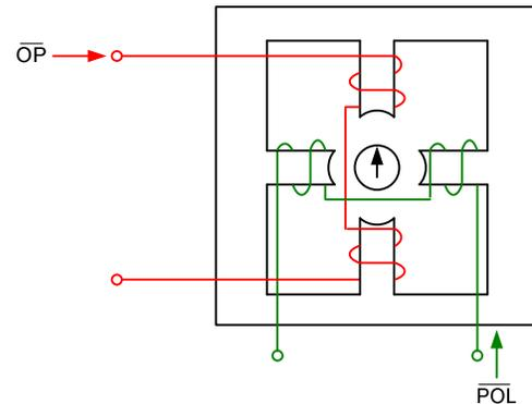
Fig. 2. Typical electromechanical induction cup relay
