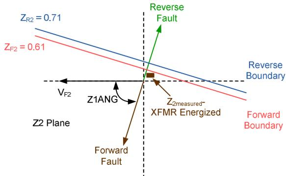
Fig. 14. A forward fault is declared with AUTO settings
