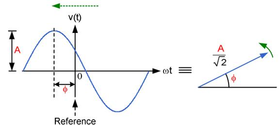
Fig. 2. Phasor representation of a sinusoidal waveform
