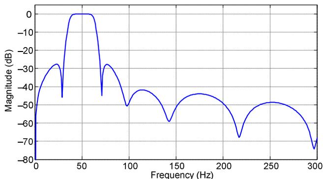
Fig. 5. Synchrophasor filter for 50 messages per second
