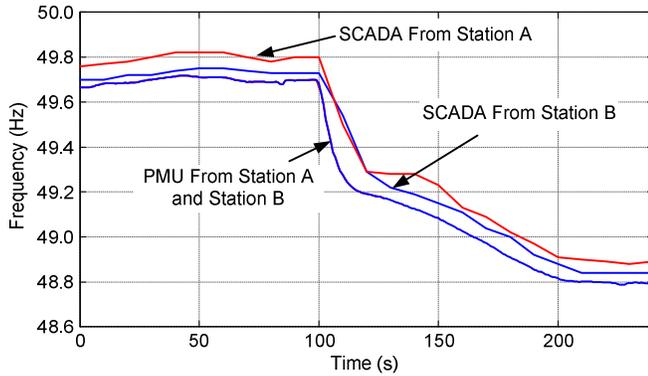
Fig. 11. Synchrophasors provide coherent frequency measurements
