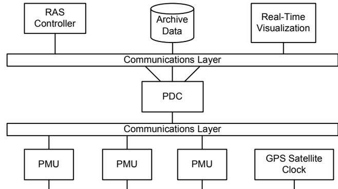
Fig. 6. Building blocks of a synchrophasor-based system
