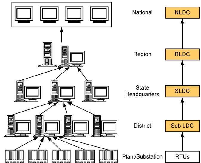
Fig. 4. Data flow from the substation to the NLDC
