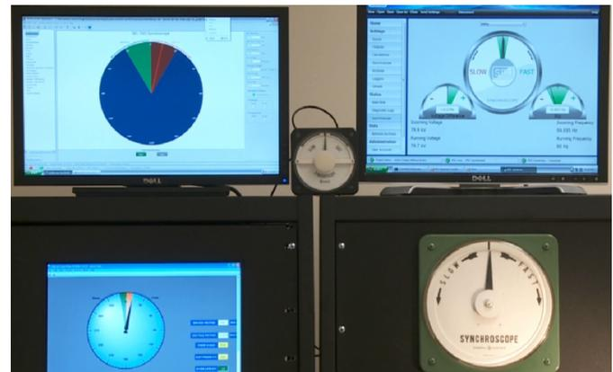
Fig. 3. Synchrophasor-based soft synchroscope test
