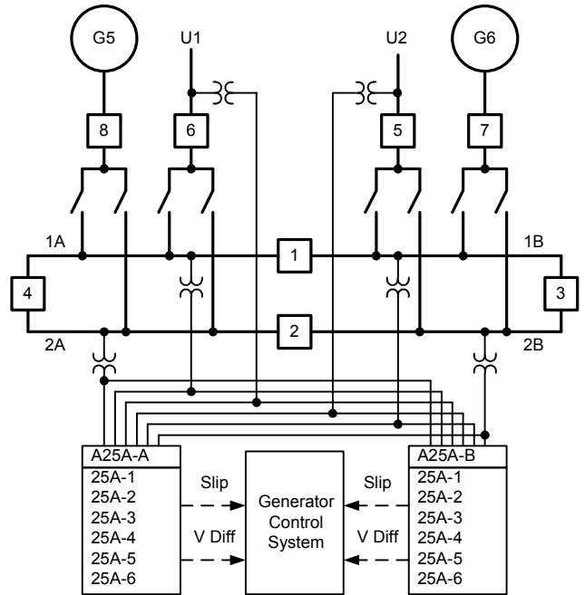
Fig. 6. Complex redundant automatic synchronizing system
