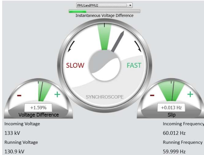
Fig. 2. Advanced PDC synchroscope
