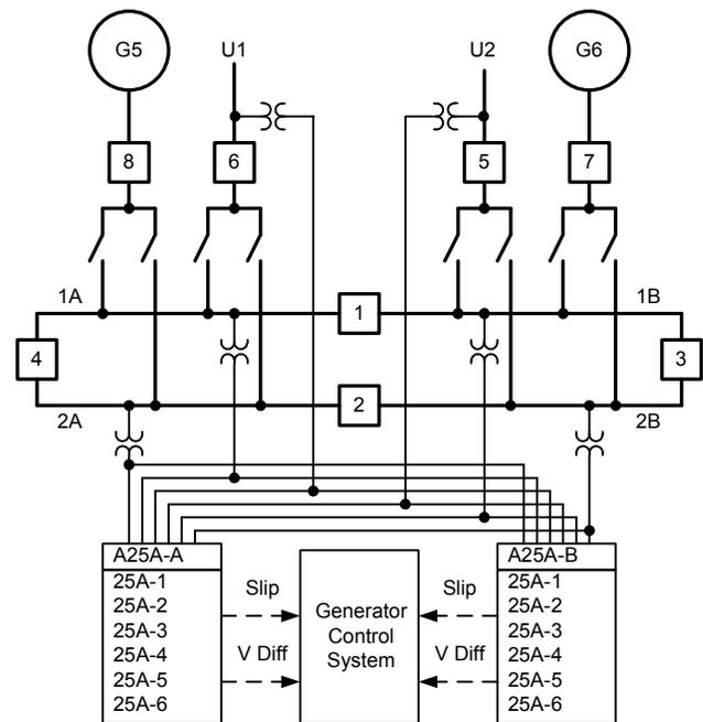
Fig. 6. Complex redundant automatic synchronizing system
