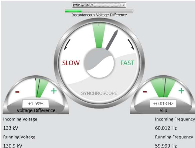
Fig. 2. Advanced PDC synchroscope
