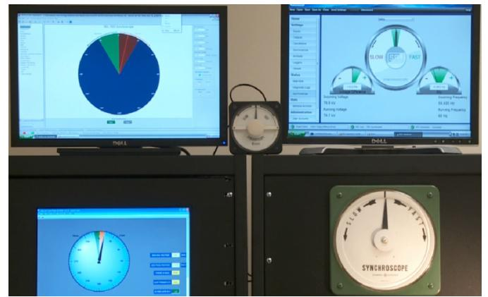
Fig. 3. Synchrophasor-based soft synchroscope test
