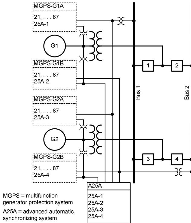
Fig. 4. Example applications using microprocessor-based automatic synchronizer(s) to eliminate VT signal switching
