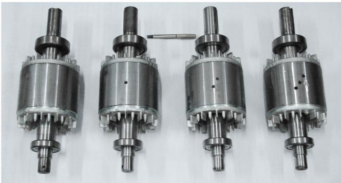
Fig. 26. Healthy rotor and rotors with one, two, and three broken bars.
