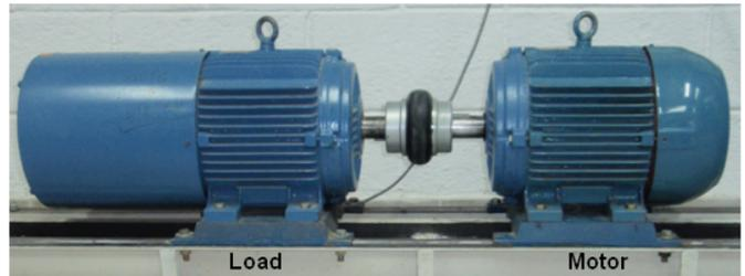
Fig. 24. Motor and its load for broken bar testing.
