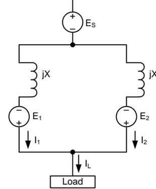
Fig. 1. Simplified two-transformer model
