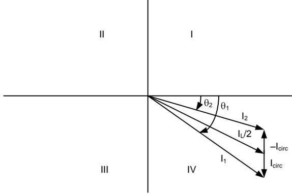
Fig. 3. Vector diagram of parallel transformer currents
