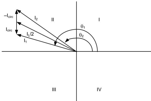
Fig. 4. Parallel transformer currents when operating in Power Quadrant II
