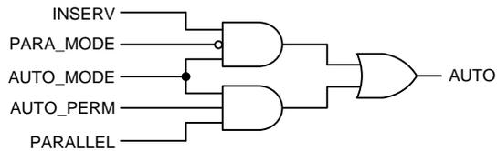
Fig. 7. Automatic mode logic
