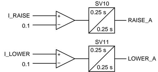
Fig. 14. Raise and lower motor current sensing
