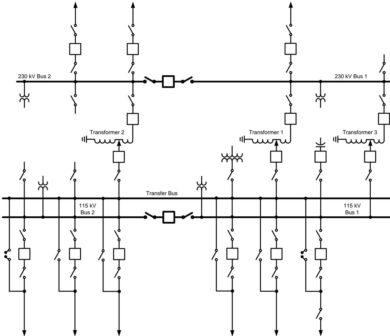
Fig. 18. Perry Road Substation one-line diagram
