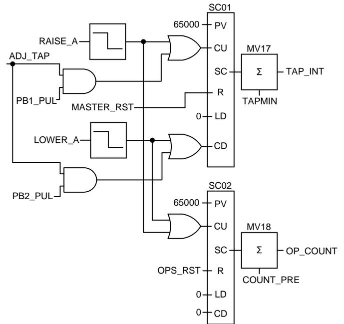
Fig. 15. Internal tap-position counter and operations counter
