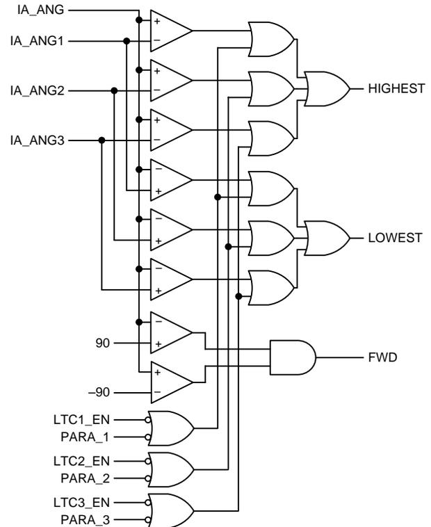
Fig. 9. Angle comparison logic
