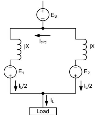
Fig. 2. Two-transformer model showing circulating current
