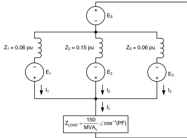
Fig. 17. Parallel transformer model
