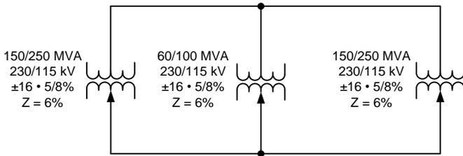
Fig. 16. Transformer arrangement used for simulation
